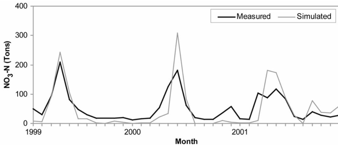
**FIGURE 8. Simulated versus measured monthly NO<sub>3</sub>-N loads at the watershed outlet during 1999-2001**
