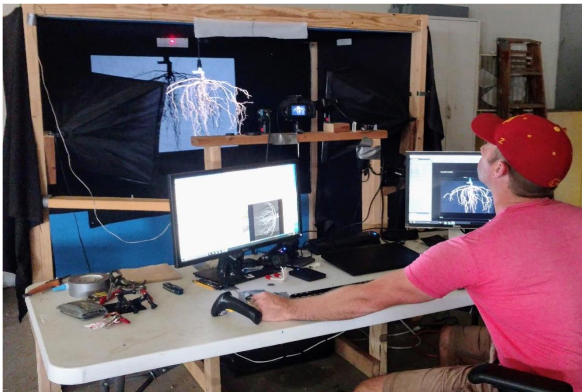
Figure 3. Soybean roots are suspended in a photo booth with images taken using multiple cameras from multiple angles.
