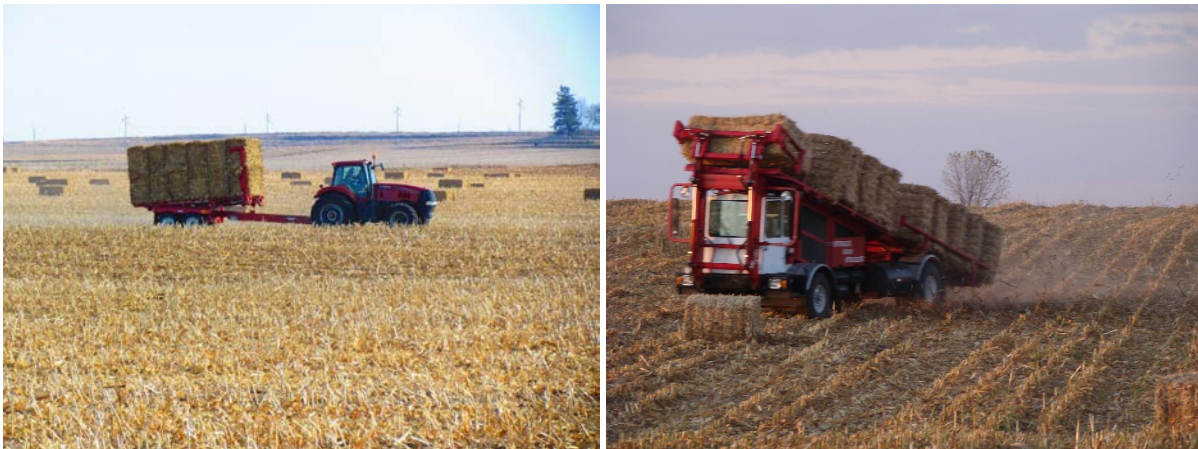
Figure 3: Stacking of bales with pull-behind (left) and self-propelled (right) stackers
