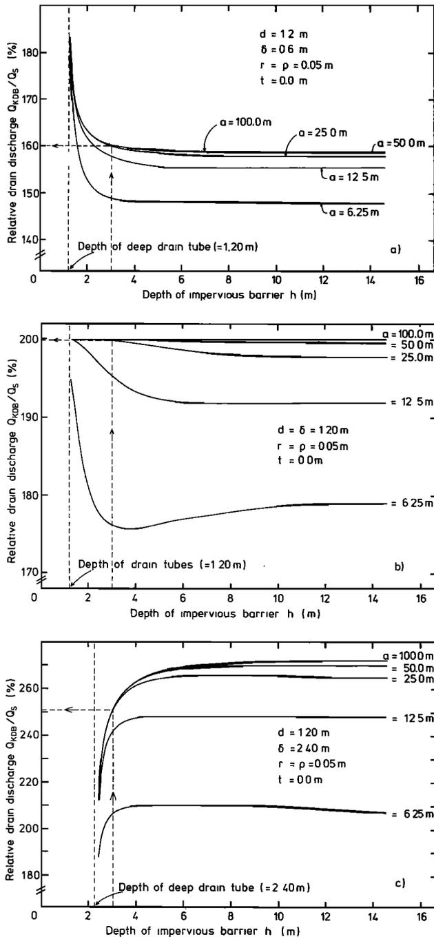
**Figure 7.** Simple nomographs to estimate the relative drain discharge  $Q_{KDB}/Q_S$  (in percent) for a dual-depth subsurface drainage system, when the depth of the single-depth tube is 1.20 m and the additional tube is (a) at 0.60 m, (b) at 1.20 m, and (c) at 2.40 m depth; other parameters are shown in the figures.
