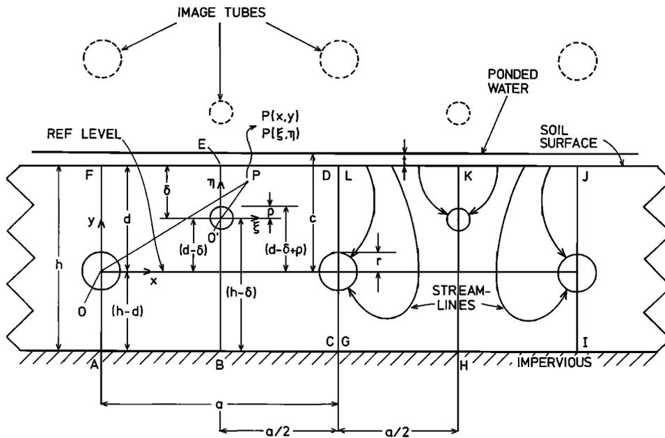
Figure 1. Geometry for dual-depth tube drainage of ponded water; only a few of the infinite number of arrays of image tubes that are implicitly used in the analysis [see Kirkham, 1949] are shown.
