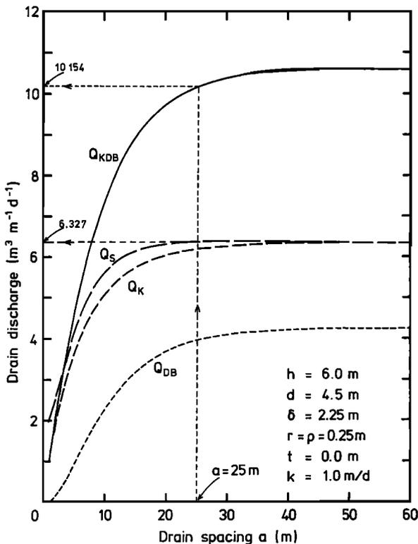
Figure 4. Dual-depth drain discharge  $Q_K$ ,  $Q_{DB}$ , and  $Q_{KDB}$  as functions of the drain spacing  $a$ ; for comparison, also the single-depth drain discharge  $Q_S$  of Kirkham [1949] is shown.
