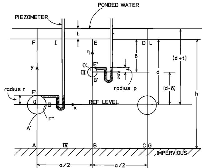
Figure 2. Boundary conditions for dual-depth drainage of ponded water.
