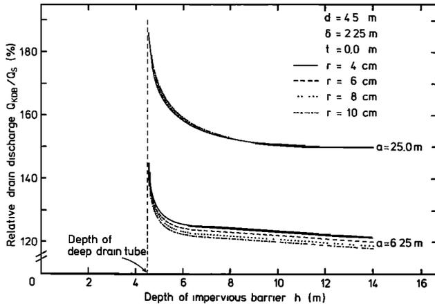
**Figure 6.** Relative drain discharge  $Q_{KDB}/Q_S$  (in percent) as a function of the depth of the impervious barrier  $h$ , for different values of the drain tube radii ( $r = \rho = 0.04, 0.06, 0.08,$  or  $0.10$  m) for two values of the drain spacing ( $a = 6.25$  or  $25.0$  m).
