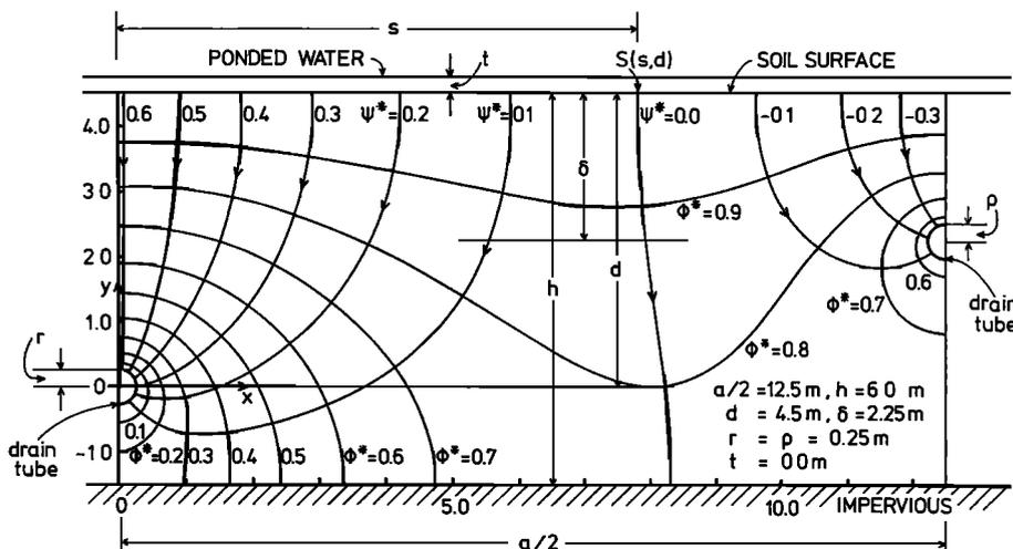
Figure 3. Flow net for a ponded-water soil that is drained by a dual-depth tube system.
