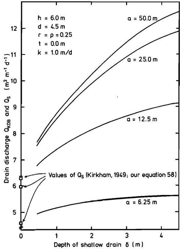
Figure 5. Dual-depth drain discharge  $Q_{KDB}$  as a function of the shallow drain depth  $\delta$  for different values of the drain spacing  $a$ ; for comparison, also the single-depth drain discharge  $Q_S$  of Kirkham [1949] is shown.
