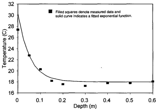
Fig. 1. The initial temperature distribution of the soil profile.
