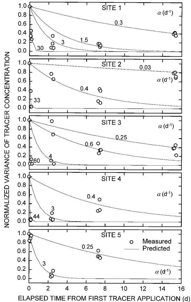
Fig. 3. The predicted and measured normalized sample variance ( $s^2(t)/s_0^2$ ) as a function of time elapsed from the start of the tracer application for each site. Here the predicted  $\alpha$  values next to the curves are derived from Eq. [10]. Note that measured  $s^2(t)/s_0^2$  values that were  $>1$  were excluded from Site 2 on the second sampling date and from Site 4 and 5 on the last sampling date.
