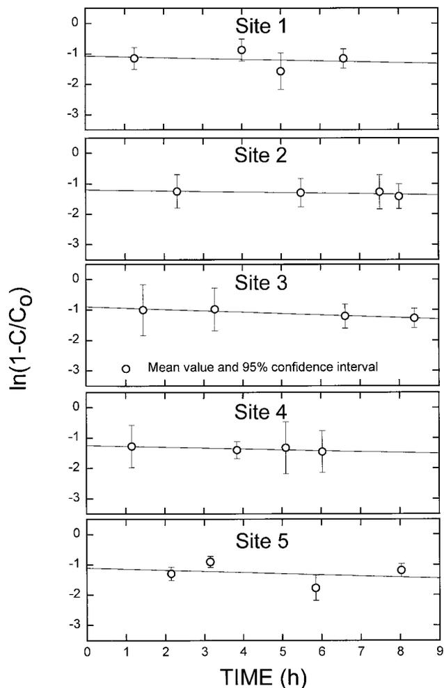
Fig. 2. Regressions of the  $\ln(1 - C/C_0)$  vs. time used by the Jaynes et al. (1995) method to estimate  $\theta_{im}$  and  $\alpha$  at each site. The slope gives  $-\alpha/\theta_{im}$  and the intercept gives  $\ln(\theta_{im}/\theta) + \ell\theta_m/(\theta_{im}q)$ .
