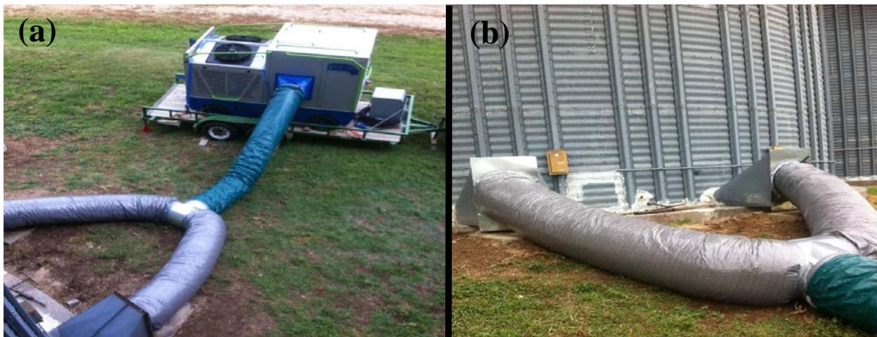
Figure 1. Grain chiller PCS-20 setup: a) Insulated duct connected to the chiller's outlet at one end and to a "T" connector at the other, b) Two ducts attached to the fan transition parts of the aeration fans that were removed.
