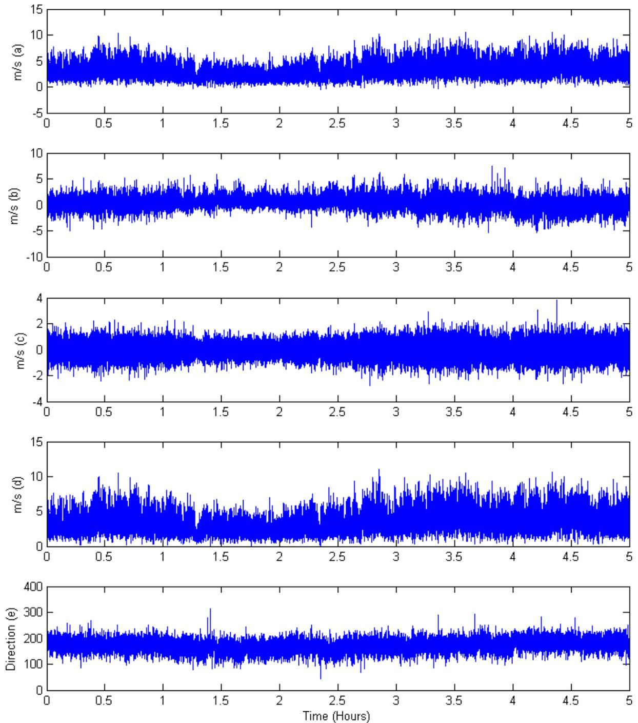
Figure 3: Data collected over a five hour period. (a) North-South, (b) East-West, (c) Vertical Wind, (d) Wind Magnitude, and (e) Wind Direction
