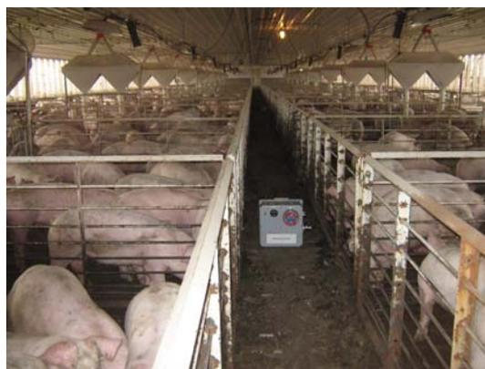
**Figure 1.** The previously developed wireless H<sub>2</sub>S detection system deployed in a swine facility prior to slurry agitation and removal.
