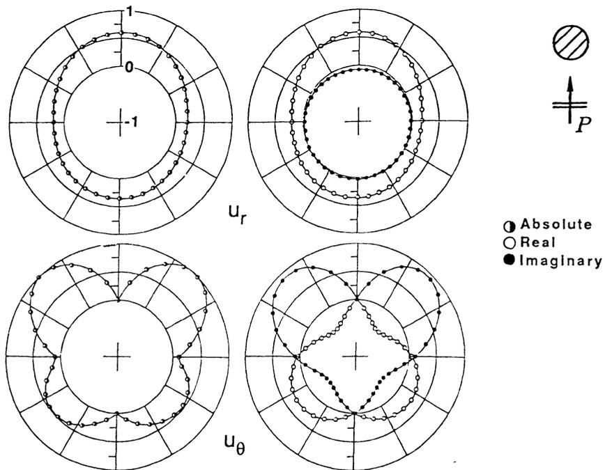
Fig.7 Radiation pattern for the case of perfect bonding.
