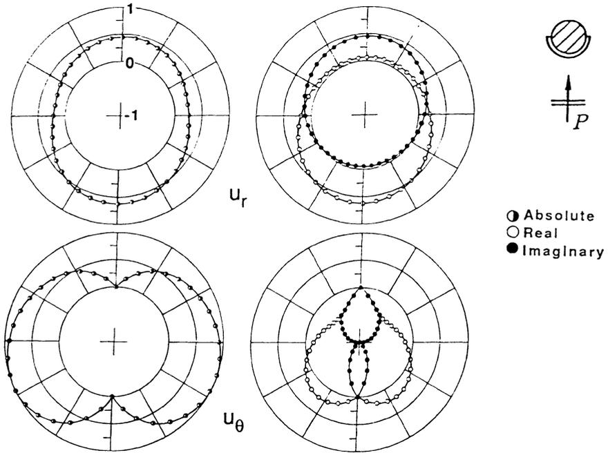
Fig.6 Radiation pattern for the case of crack at insonified side.
