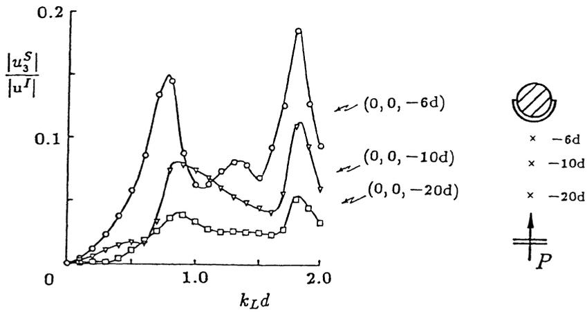
Fig.2 Scattered field amplitudes  $|u_3^S|/|u^i|$  vs. wave number  $k_L d$ .
