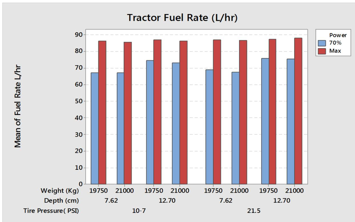
**Figure 6.** Mean fuel rate of tractor with standard and added weight.
