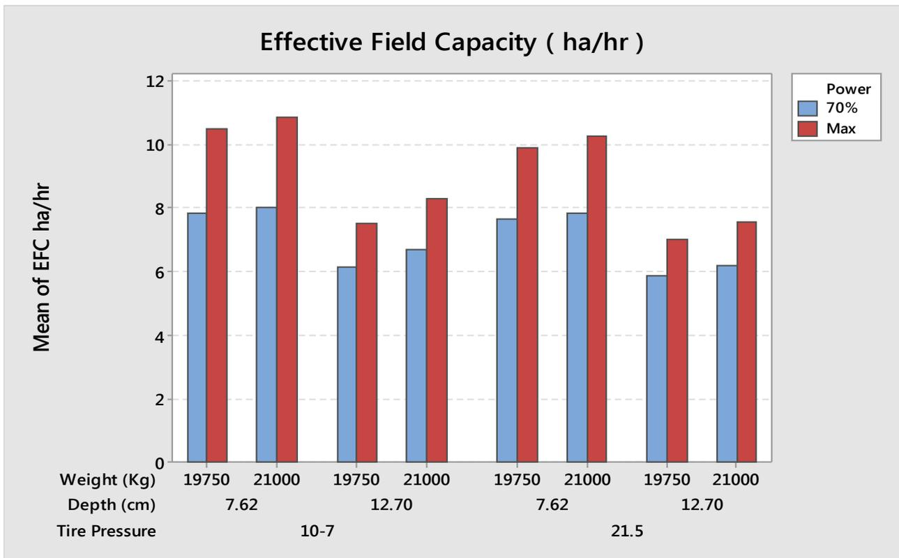
**Figure 8.** Mean effective field capacity of tractor with standard and added weight.
