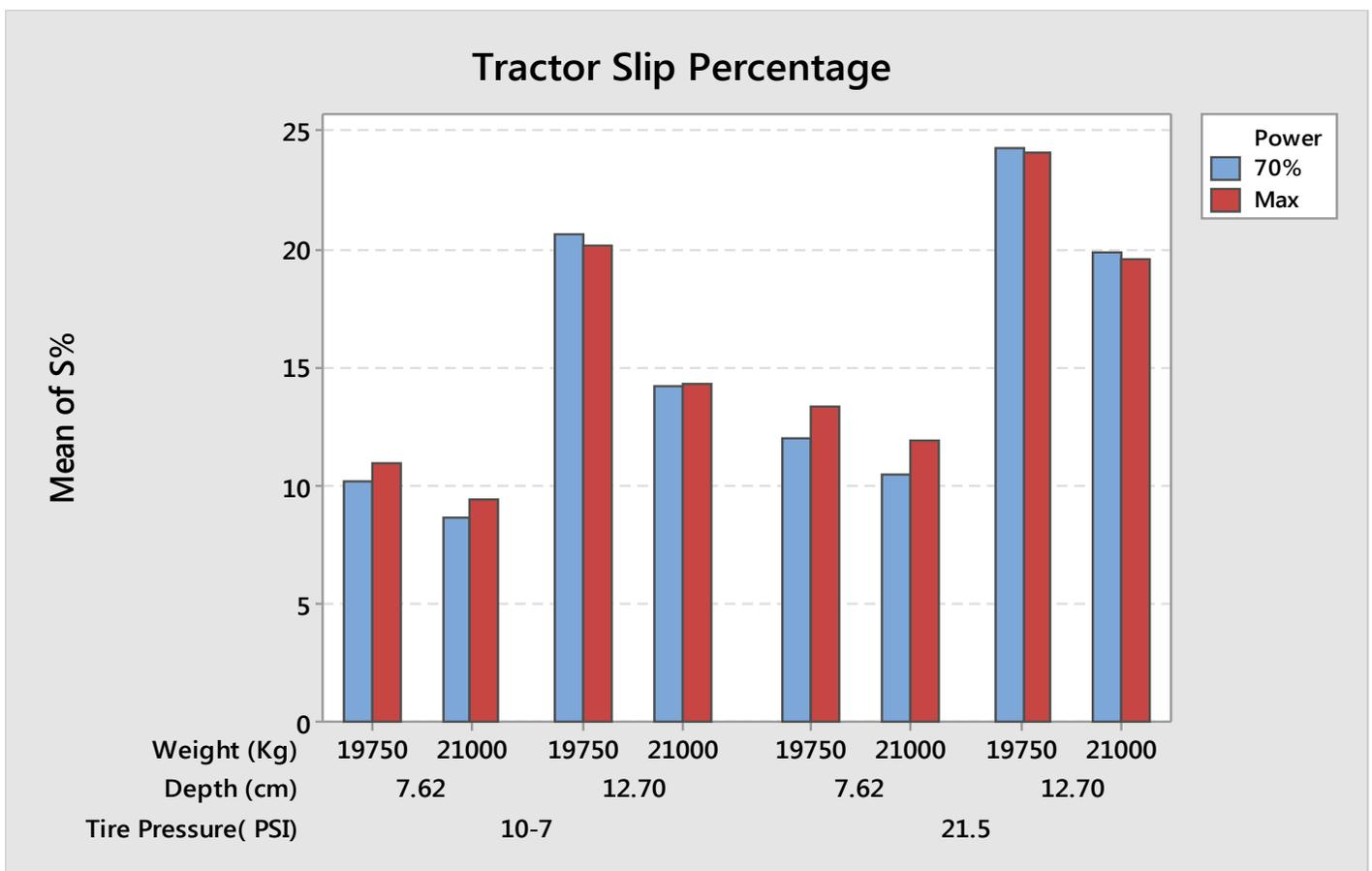
**Figure 7.** Mean slippage percentage of tractor with standard and added weight.
