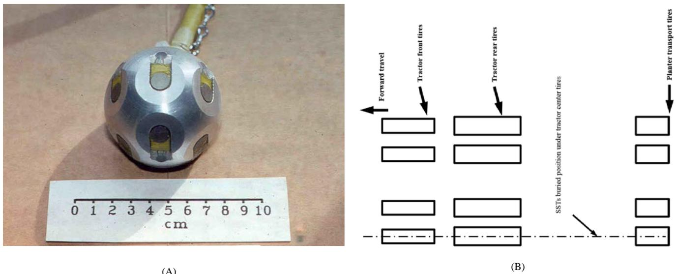
**Figure 2. (A) Soil State Transducers (SSTs) used in the experiment (six axis 345 kPa pressure sensors) and (B) position of SSTs buried beneath the centerline of the path of the outer left tractor and planter transport tires. The SSTs were buried at 15-cm and 30-cm beneath the untrafficked soil surface.**
