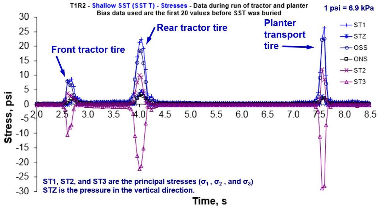
Figure 4. Soil stress states calculated from SSTs pressure data. ST1, ST2, ST3 are the principal stresses (sigma-1, sigma-2, sigma-3) and STZ vertical stress. ONS is Octahedral Normal Soil Stress and OSS is Octahedral Shear Soil Stress.
