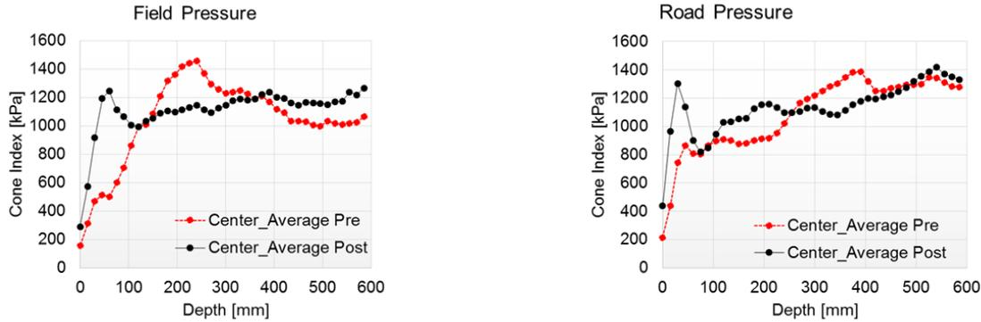
Figure 7. Soil cone index from tire centerline position for “field”(low) and “road” (high) tire inflation pressures. (sample size, n = 3 for each cone index profile).
