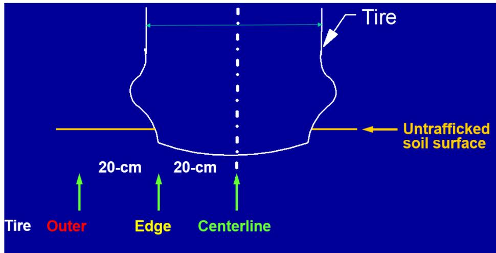
Figure 3. Soil cone index measurement sampling positions for before and after tire passes.
