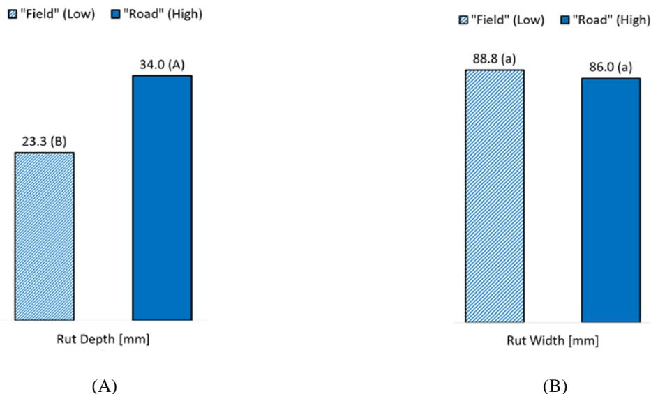
Figure 11. Soil rut depth (A) and soil rut width (B) from “field” (low) and “road” ( high) tire inflation pressure after tractor-planter pass ( sample size , n = 9 for each treatment factors). For each variables (soil rut depth and soil rut width), similar letter indicate no statistical differences at P-value = 0.01.
