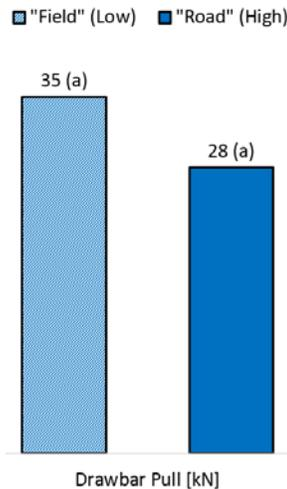
Figure 10. Tractor-planter drawbar pull for “field” (low) and “road” ( high) tire inflation pressure. Similar letter indicate no statistical differences at P-value = 0.01. P-value 0.0715 (sample size, n = 3 for each treatment factors).
