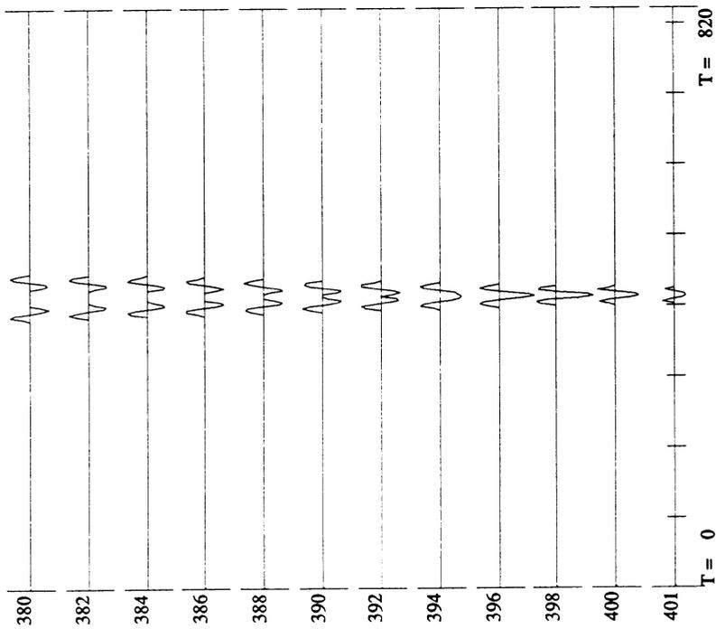
Fig. 6 — Detailed representation of the reflection of a sine wave by the bottom surface of the material. The parameters used in this plot are  $\alpha = \beta = 20$ ,  $\tau = 5$  ns and  $\epsilon = 31.75 \mu$ .
