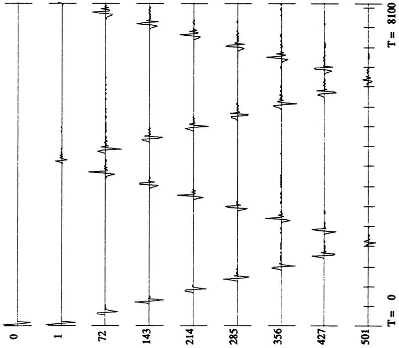
Fig. 4 — Propagation of a sine wave. The parameters used in this plot are  $\alpha = 25$ ,  $\beta = 100$ ,  $\tau = 1$  ns and  $\epsilon = 25.4 \mu$ .
