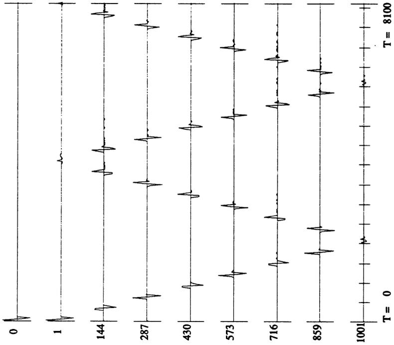
Fig. 3 — Propagation of a sine wave. The parameters used in this plot are  $\alpha = 50$ ,  $\beta = 100$ ,  $\tau = 1$  ns and  $\epsilon = 12.7 \mu$ .
