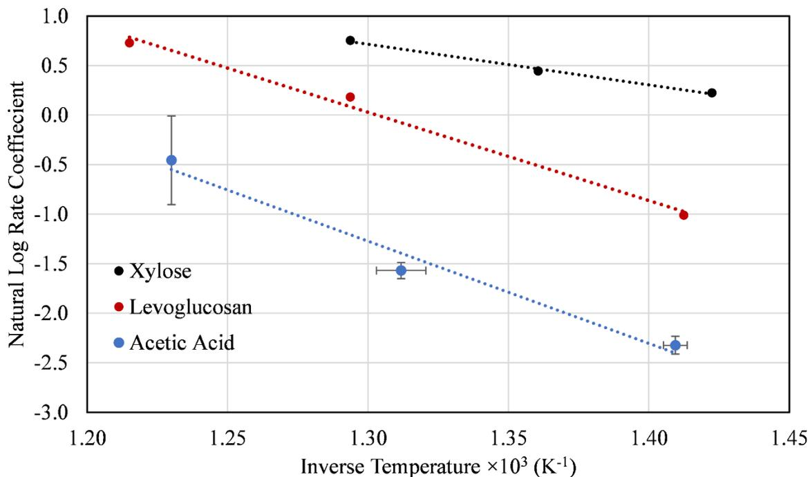
**Figure 5.** Arrhenius plot of the global oxidation rates of the three-ideal bio-oil components. Error bars on the acetic acid trials are the sample standard deviation from replicate trials and the average internal temperature for each trial. Note: levoglucosan and xylose only had single trials performed.
