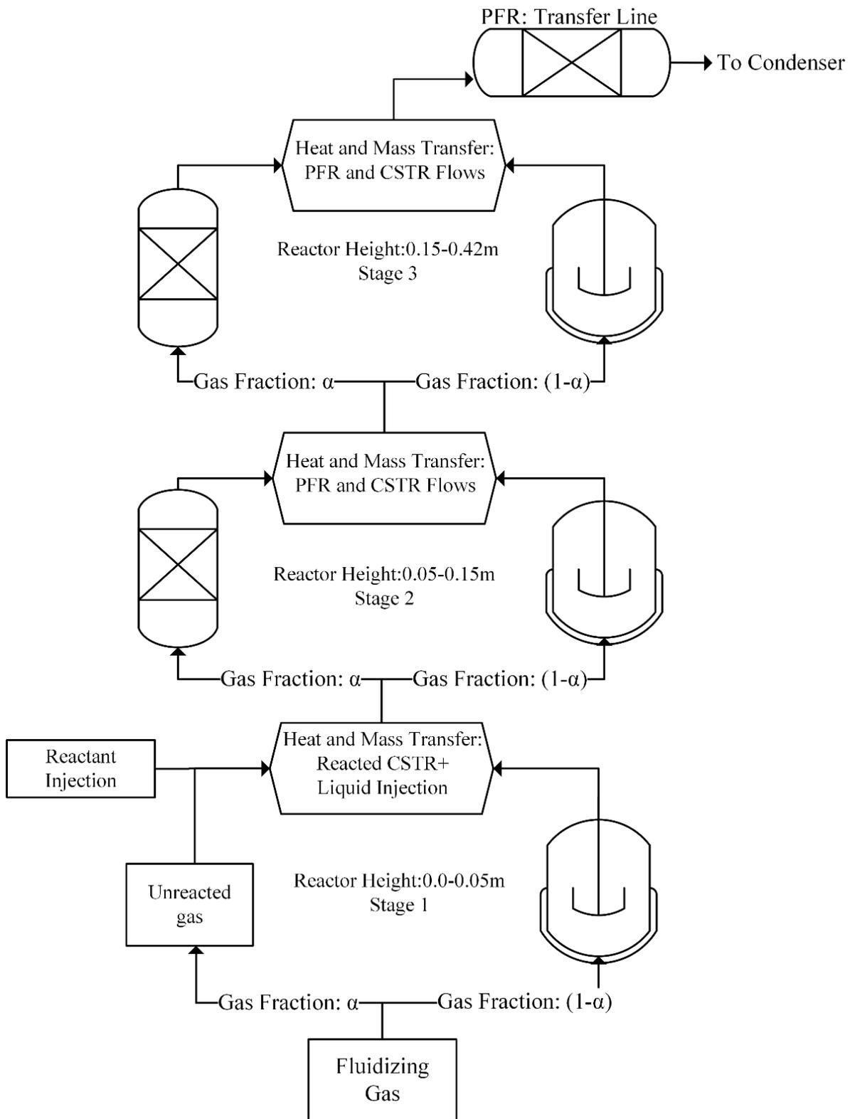
**Figure 4.** Two-phase theory calculations indicated three stages were necessary to model the bubbling fluid bed reactor. The first stage is just a CSTR with no PFR to account for back mixing of the liquid reactant and fluidizing gas.
