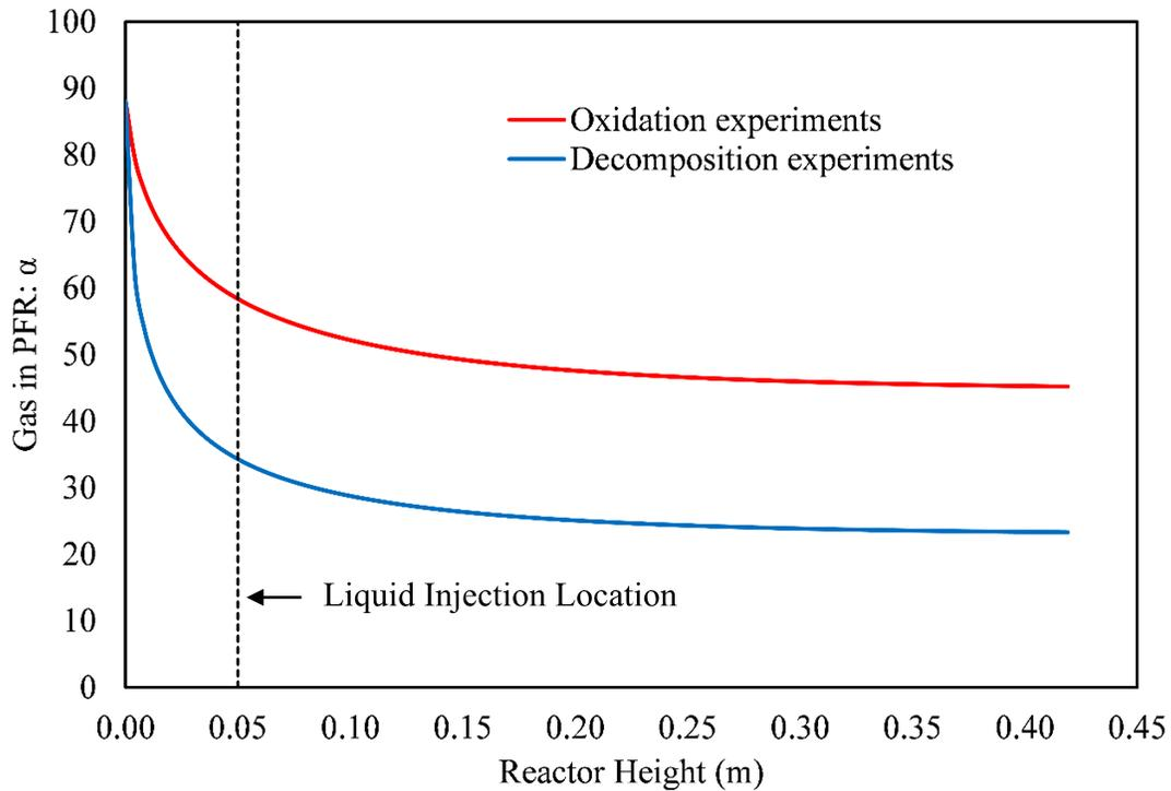
**Figure 3.** Gas percentage allocated to the PFR versus reactor height for typical operating conditions in oxidation and decomposition studies. The dashed line at 0.05m indicates location of liquid injection. For the decomposition experiments, the average sand particle size was 300  $\mu\text{m}$  with a fluidizing gas flow rate of 3.5 SLPM of nitrogen. The oxidative experiments utilized 600  $\mu\text{m}$  sand with 8 SLPM of nitrogen and 4 SLPM of air.
