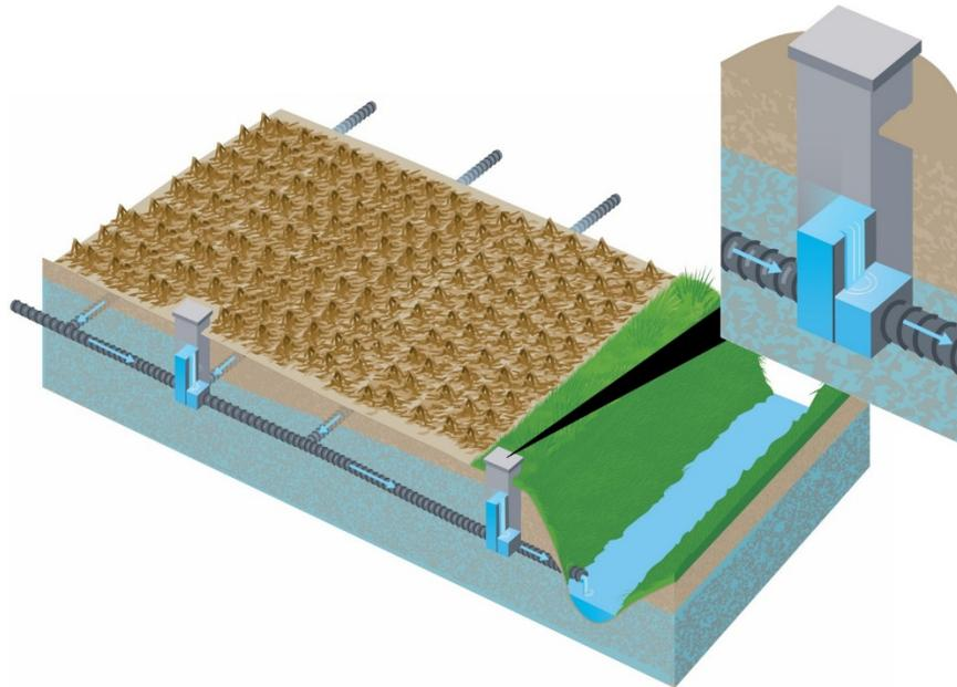
**Figure 1. Controlled drainage consists of water control structures which manage the soil water table depth. Multiple control structures are used to manage a relatively even subsurface water table across variable surface topography.**
