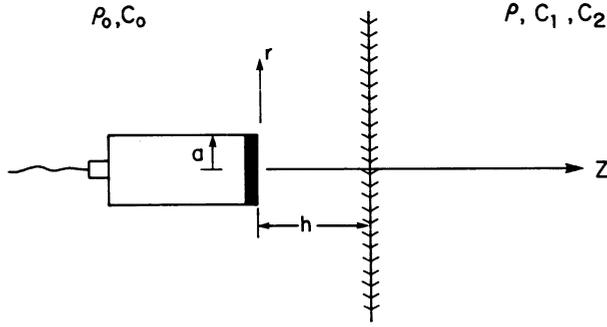
Fig. 1. Immersion transducer geometry.
