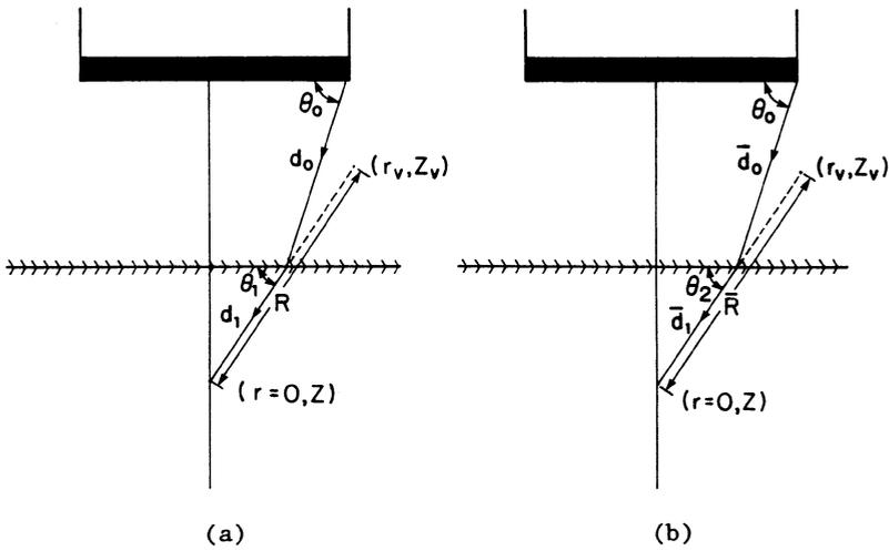
Fig. 3. Ray paths corresponding to (a) P-waves in the solid (b) shear waves in the solid.
