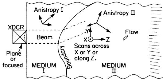
Figure 1 A diagram showing the operation of the Newberry-Thompson measurement model with its versatile capabilities.
