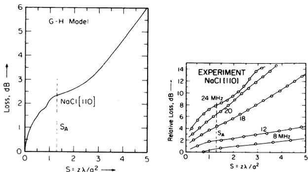
Figure 8 G-H model used to explain the experimental data on ultrasonic loss in the [110] direction in NaCl.
