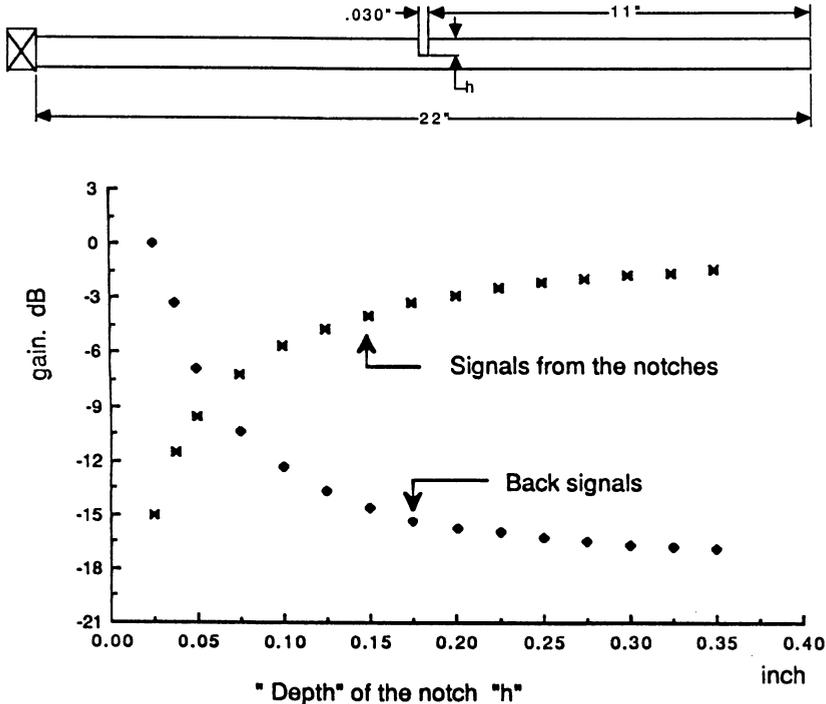
Figure 2. Dependence of Signal Amplitude on Notch Depth.
