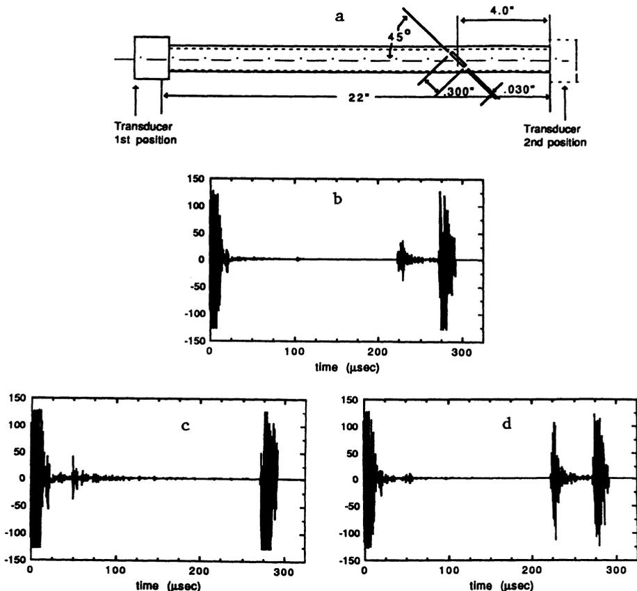
Figure 1. Inspection of EDM Notches of Different Orientations:
