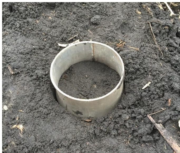
Figure 1. Ring used to take bulk density core samples which was driven in with a hammer and wood plank.
