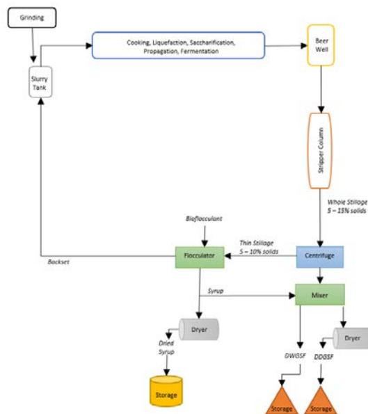
**Figure 01.** Flow chart of a corn-based ethanol plant utilized for investigate LCA and TEA considering the flocculation process for wastewater.
