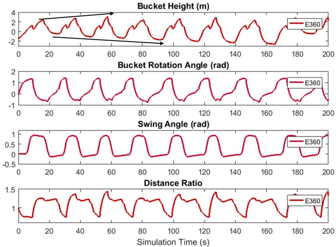
**Figure 4. Machine response of the closed loop simulation by indicating increasing trench depth and pile height during simulation. Arrows on the Bucket Height graph demonstrate the increasing pile height and trench depth.**
