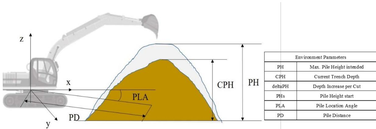
**Figure 2. Pile model to represent the increasing trench depths during the operation.**
