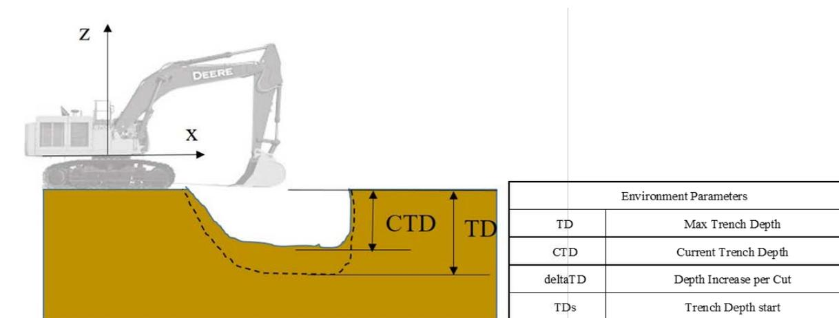
**Figure 3. The trench model to represent the increasing trench depths during the operation.**
