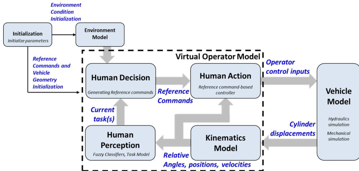
**Figure 1. Virtual operator model structure consists of several models representing human information processing.**
