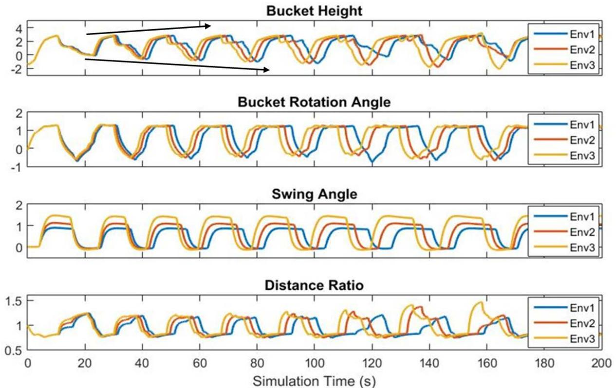
**Figure 5. Machine Response of the Closed Loop Simulation using different Environment Situation Setting. Arrows on the Bucket Height graph demonstrate the increasing pile height and trench depth.**
