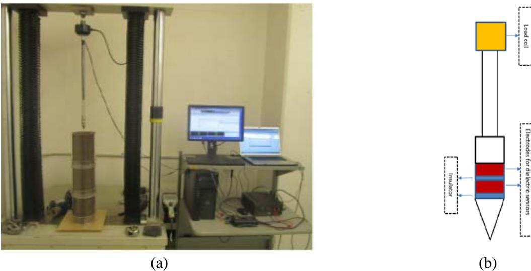
**Fig 1: Soil preparation and cone index measurement in the laboratory: (a) three soil layers; (b) cone penetrometer probe with multiple sensors for measurement of penetration forces and moisture content.**
