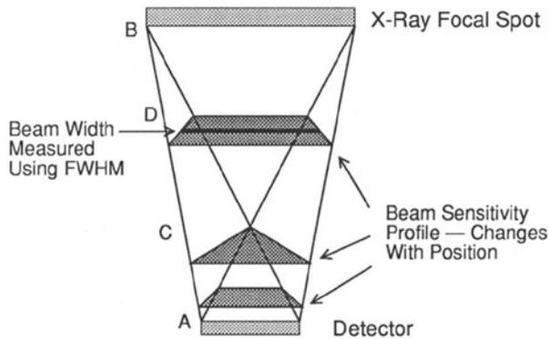
Figure 1. The drawing illustrates the beam sensitivity profile for different positions along the beam path.
