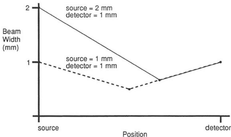
Figure 3. The graph shows beam width as a function of position between the source and detector for two focal spot sizes.
