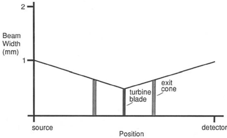
Figure 4. The graph shows the beam width as the beam passes through a turbine blade and an exit cone when the geometry is optimized for the turbine blade.
