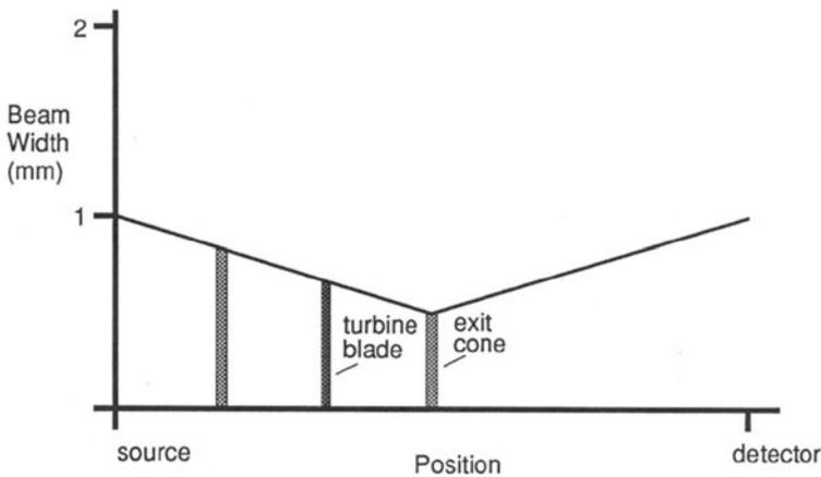
Figure 5. The graph shows the beam width as the beam passes through a turbine blade and an exit cone when the geometry is optimized for the exit cone.
