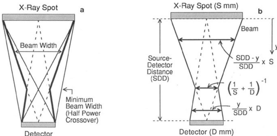
Figure 2. Drawing a shows the beam width obtained by plotting the FWHM lines; drawing b gives formulas for the beam width in different regions of the beam path.
