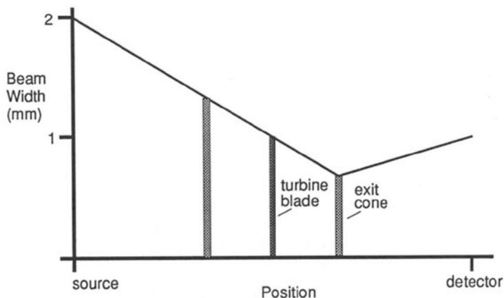
Figure 6. The graph shows the beam width as the beam passes through a turbine blade and an exit cone when an x-ray source with a 2 mm focal spot is used.
