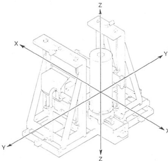
Figure 7. The drawing shows the mechanical configuration of ACTIS. The source tower on the left, which holds up to three x-ray sources, and the detector tower on the right both move along the y axis to vary the scanner geometry.
