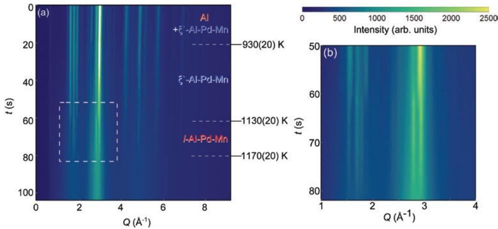
**Fig. 6:** The azimuthally integrated HEXRD patterns taken on heating the Al–Pd–Mn sample. Panel (a) shows the full temperature/time range of the measurement. Dashed lines indicate the temperatures where phases disappear in the diffraction pattern. Panel (b) displays an expanded view of the temperature and momentum transfer range enclosed by the box in panel (a), where the orthorhombic  $\xi'$ -phase transforms to the  $i$ -phase and then fully melts.
