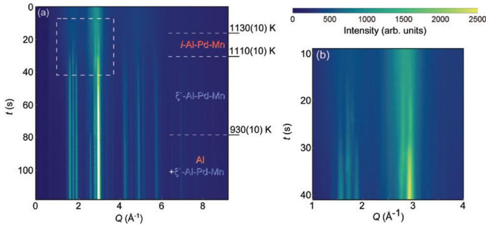
**Fig. 3:** The azimuthally integrated HEXRD patterns taken on free-cooling the Al–Pd–Mn sample. Panel (a) shows the full temperature/time range of the measurement. The intensity is color-coded. Dashed lines indicate the temperatures at which phases appear in the pattern. Panel (b) displays an expanded view of the temperature and momentum transfer range enclosed by the box in panel (a), where the liquid transforms to the  $i$ -phase and then to the orthorhombic  $\xi'$ -phase.
