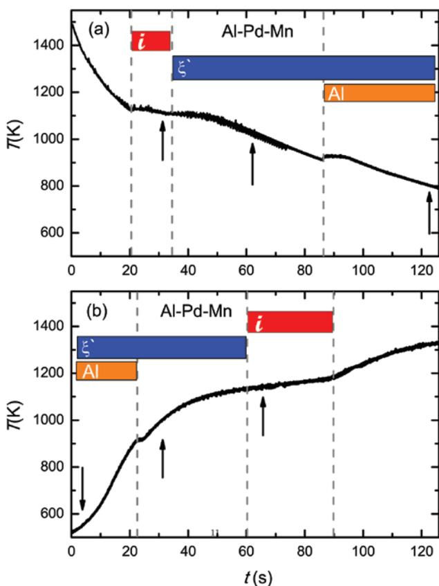
**Fig. 2:** The (a) cooling and (b) heating curves of the Al–Pd–Mn sample as described in the text. The phases and transition temperatures were identified from the x-ray diffraction patterns and are labeled by the colored bars above the curve. The arrows denote the temperatures for the x-ray diffraction data shown in Figs. 5 and 7.
