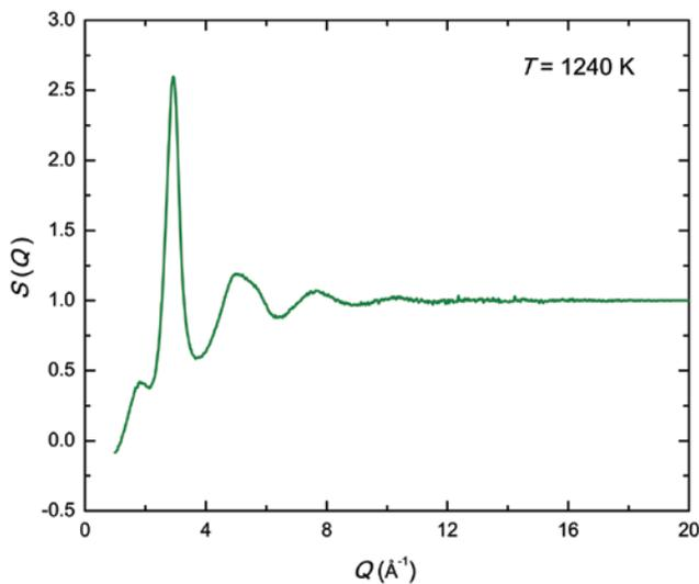
**Fig. 4:** The liquid structure factor,  $S(Q)$ , derived from the HEXRD data measured at  $T=1240$  K, which is 100 K above the appearance of the  $i$ -phase in the sample.
