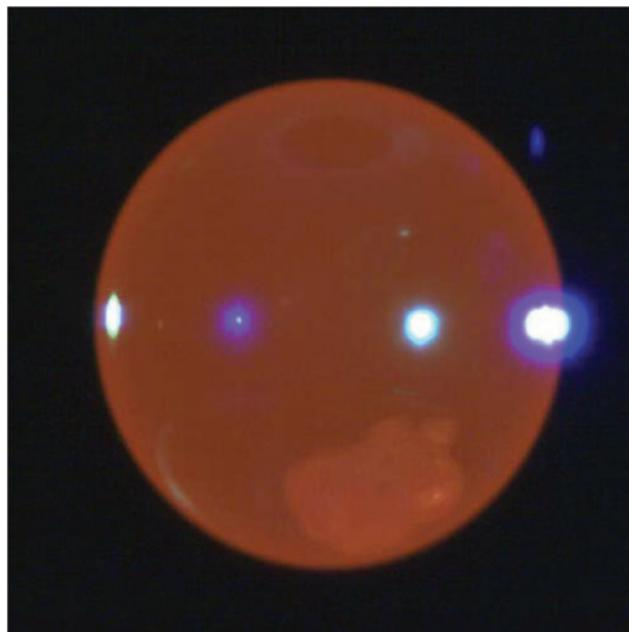
**Fig. 1:** A view of the liquid sample taken during a heating cycle in the ISU-ESL. The bright spots are reflections of the positioning LEDs. A small translucent patch of  $\text{Al}_2\text{O}_3$  on the surface of the alloy can be seen in the lower right quadrant of the sphere.
