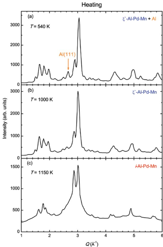
**Fig. 7:** The azimuthally integrated diffraction patterns from the Al–Pd–Mn sample during heating at selected temperatures. The diffraction pattern at (a)  $T=540$  K and (b)  $T=1000$  K closely reproduce those in the same temperature regimes on free-cooling. (c) The diffraction data at  $T=1020$  K were taken just as the icosahedral phase reappears.
