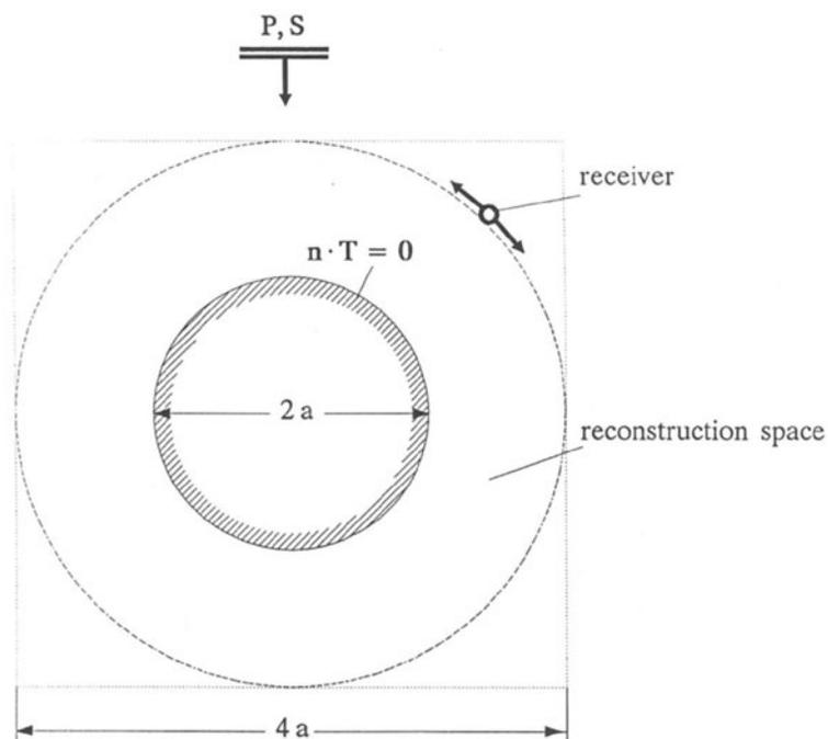
Figure 7. Bistatic multifrequency experiment  $0 \leq k_P a \leq 40.$ ,  $k_P = \frac{\omega}{c_P}$ ,  $c_P = 5900 \frac{m}{s}$ ,  $c_S = 3200 \frac{m}{s}$
