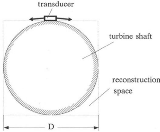
Figure 3. Monostatic multifrequency experiment  $f_0 = 4.3\text{MHz}$  ,  $c_P = 5920\frac{\text{m}}{\text{s}}$  ,  $D = 369\text{mm}$ , P-P mode
