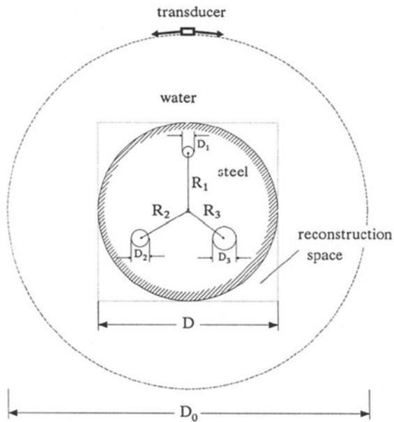
Figure 5. Monostatic multifrequency experiment  $f_0 = 2.25 \text{ MHz}$  ,  $c_{P,water} = 1480 \frac{m}{s}$  ,  $c_{P,steel} = 5690 \frac{m}{s}$  ,  $D = 80mm$  ,  $D_0 = 148mm$   $D_1 = 2mm$ ,  $D_2 = 4mm$ ,  $D_3 = 6mm$ ,  $R_1 = 30mm$ ,  $R_2 = 25mm$ ,  $R_3 = 20mm$  , P-P mode
