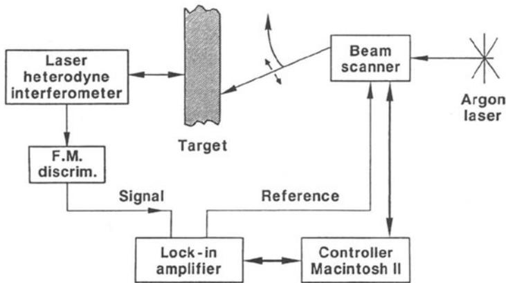
Figure 1. Block diagram of photoacoustic laser scanning and interferometer detection system.
