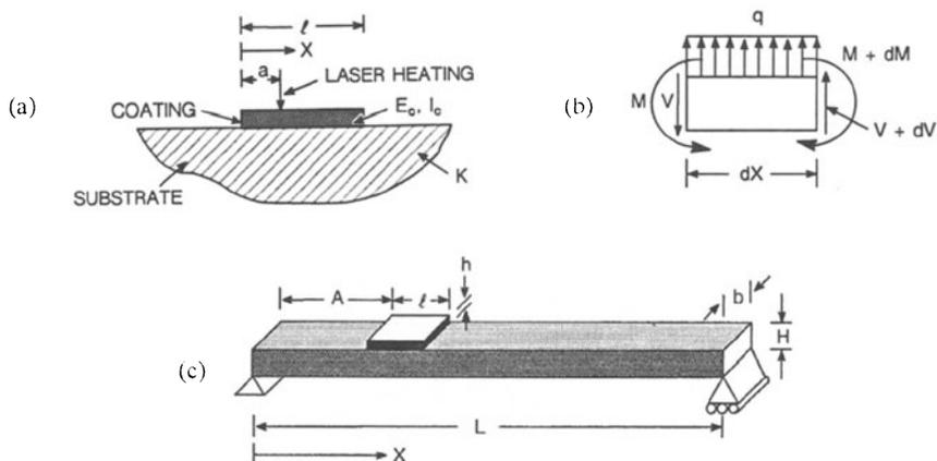
Figure 2. Thermomechanical beam model used for the analysis.
