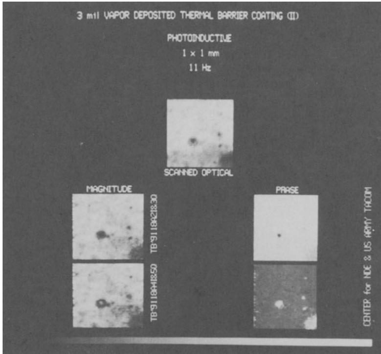
Fig. 4. Images of a small pore in an yttria-stabilized zirconia thermal barrier coating 75  $\mu\text{m}$  thick on a nickel alloy substrate. Area imaged is 1 x 1 mm. At the top is a scanned optical image, at the bottom are photoinductive magnitude (left) and phase (right) images from two different lock-in amplifiers.
