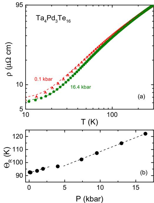
FIG. 9. (a) Data (symbols) and Bloch-Grüneisen-Mott fits (see the text) for  $\rho(T)$  data taken at 0.1 and 16.4 kbar; (b) pressure dependence of the Debye temperature,  $\Theta_R$ , obtained from the fits. Dashed lines are guides for the eye. The error bars for the values of  $\Theta_R$  obtained as a result of fits are  $\leq 1.1$  K, i.e., smaller than the size of the symbols.
