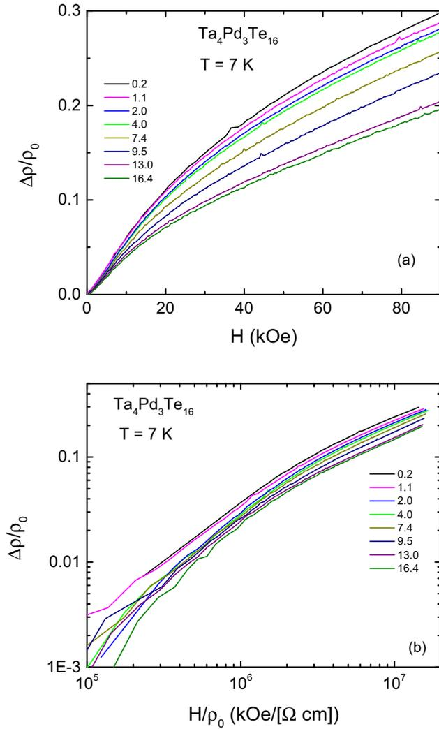
FIG. 10. (a) Normal state, low temperature ( $T = 7$  K) magnetoresistivity of  $Ta_4Pd_3Te_{16}$  plotted as  $\Delta\rho/\rho_0 = (\rho_H - \rho_{H=0})/\rho_{H=0}$  vs  $H$ . Data from the panel (a) presented on a Kohler plot,  $\Delta\rho/\rho_0$  vs  $H/\rho_0$ , on a log-log scale.
