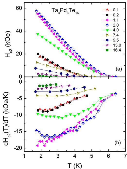
FIG. 6. (a) Temperature dependent upper critical field [ $H \parallel (-1\ 0\ 3)$ ] measured at different pressures (pressure values are given in kbar). (b) Corresponding derivatives,  $dH_{c2}/dT$ , at different pressures. The error bars are less than the size of the symbols.
