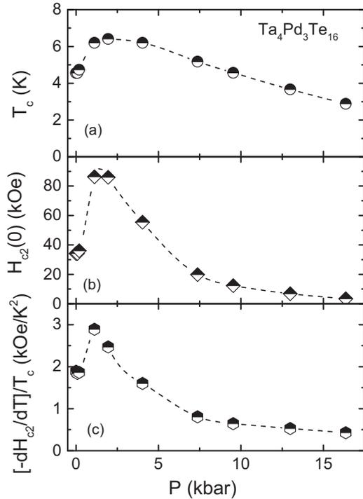
FIG. 7. Pressure dependences of (a) superconducting transition temperature; (b) extrapolated to  $T = 0$  K upper critical field [for  $H \parallel (-1\ 0\ 3)$ ]; (c) temperature derivatives of the upper critical field (taken at  $T = 2$  K) normalized by the  $T_c$ ,  $[-dH_{c2}/dT]/T_c$ . The error bars are smaller than the size of the symbols.
