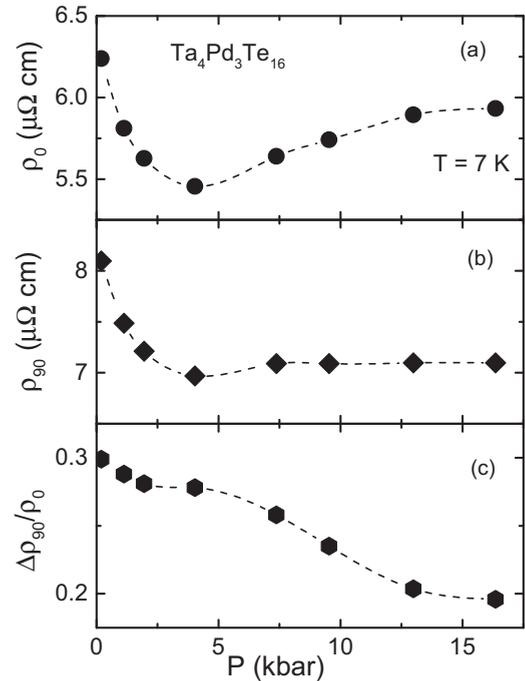
FIG. 11. Pressure dependence of (a) zero field resistivity,  $\rho_0$ , (b) resistivity in  $H = 90$  kOe magnetic field,  $\rho_{90}$ , and (c) magnetoresistivity,  $\Delta\rho_{90}/\rho_0 = (\rho_{H=90\text{ kOe}} - \rho_{H=0})/\rho_{H=0}$ , measured at  $T = 7$  K. The error bars are smaller than the size of the symbols. Dashed lines are guides for the eye.
