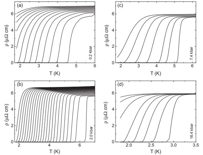
FIG. 5. Examples of low temperature  $\rho(T)$  curves measured at different applied magnetic fields and at different pressures. (a)  $P = 0.2$  kbar,  $0 \leq H \leq 30$  kOe, steps 2.5 kOe; (b)  $P = 2.0$  kbar,  $0 \leq H \leq 57.5$  kOe, steps 2.5 kOe; (c)  $P = 7.4$  kbar,  $H = 0, 1.25$  kOe,  $2.5 \leq H \leq 12.5$  kOe, steps 2.5 kOe; (d)  $P = 16.4$  kbar,  $0 \leq H \leq 1$  kOe, steps 0.25 kOe,  $1 \leq H \leq 2.5$  kOe, steps 0.5 kOe.
