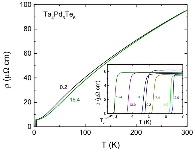
FIG. 3. Zero field resistivity of  $\text{Ta}_4\text{Pd}_3\text{Te}_6$  at  $\sim 0.2$  kbar and  $\sim 16.4$  kbar (at low temperature) pressure. Inset: resistive superconducting transitions at several selected pressures (values in kbar are given). Offset criterion for  $T_c$  is shown for the 16.4 kbar data in the inset.
