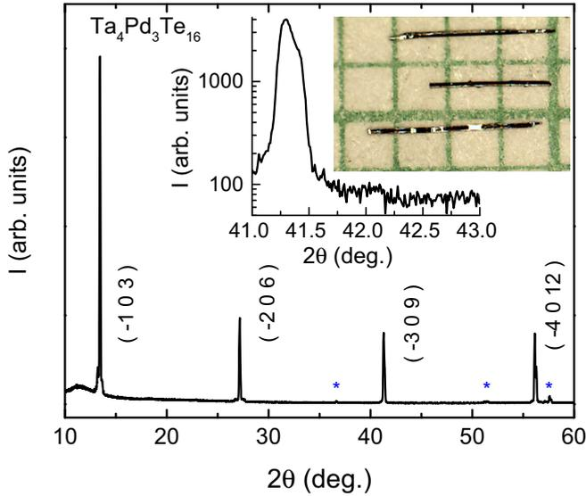
FIG. 1. Single crystal XRD pattern for  $\text{Ta}_4\text{Pd}_3\text{Te}_{16}$ . Blue stars mark Te flux peaks. Insets: part of the diffraction pattern between  $41^\circ$  and  $43^\circ$ , around  $(-3\ 0\ 9)$  peak on a semilog plot, and typical crystal picture over a mm scale.
