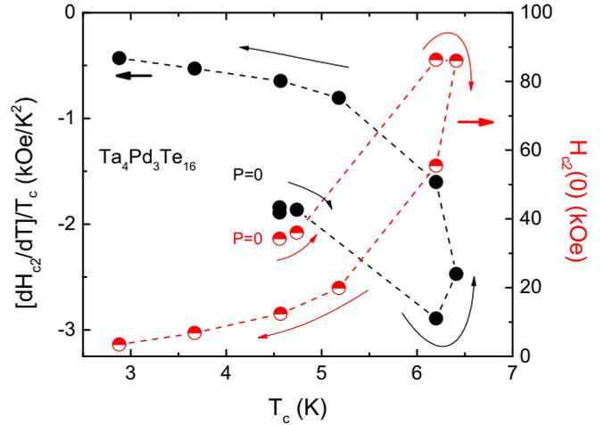
FIG. 8. Normalized temperature derivative of the upper critical field (left Y-axis), and extrapolated to  $T = 0$  K upper critical field, plotted as a function of  $T_c$ . Arrows indicate the directions of increasing pressure for each manifold. The error bars are smaller than the size of the symbols.
