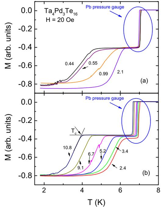
FIG. 2. Subset of zero-field-cooled temperature-dependent magnetization data measured at different pressures (values in kbar are given in the plot). Each curve contains a signal from the  $\text{Ta}_4\text{Pd}_3\text{Te}_{16}$  sample and the Pb pressure gauge. Onset criterion for  $T_c$  is shown for the 10.8 kbar data. Panel (a): lower pressure range with  $T_c$  increasing with increasing pressure; panel (b): higher pressure range with  $T_c$  decreasing with increasing pressure.
