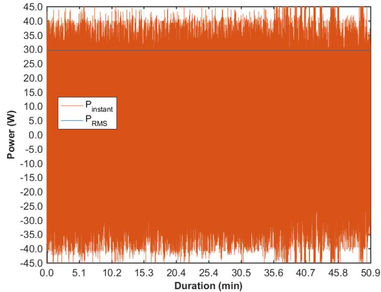
**Figure 3. Example of instantaneous power measurement and calculated Root-Mean Square (RMS) power for test 2 during the steady-state period. The RMS power was compared with the theoretical heat loss predicted from TESA measurements and a Simulink model.**
