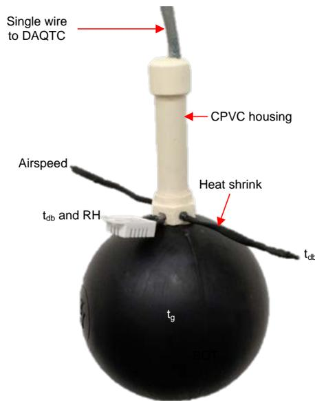
**Figure 1. Image of a Thermal Environment Sensor Array (TESA) featuring dry-bulb temperature ( $t_{db}$ ), relative humidity (RH), airspeed, and Black Globe Thermometer (BGT) sensors. Globe temperature ( $t_g$ ) is obtained from a  $t_{db}$  sensor at the center of the BGT and used to calculate mean radiant temperature ( $t_{mr}$ ).**
