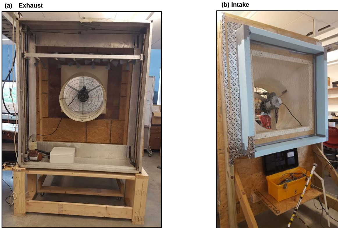
Figure 4. Measurement of airflow from a 61 cm (24 in.) fan with a discharge cone (a) FANS unit measuring exhaust airflow and (b) SWEAP measuring the intake airflow
