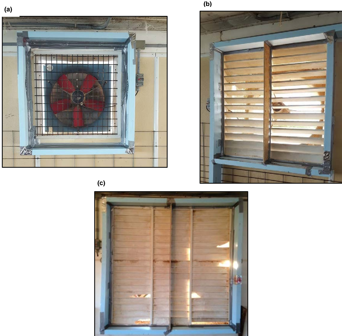
Figure 5. Field testing: blue board frame encompassing a (a) 61 cm (24 in.) fan with a hood and (b) 91 cm (36 in.) fan with a cone (c) 122 (48 in.) fan with a cone
