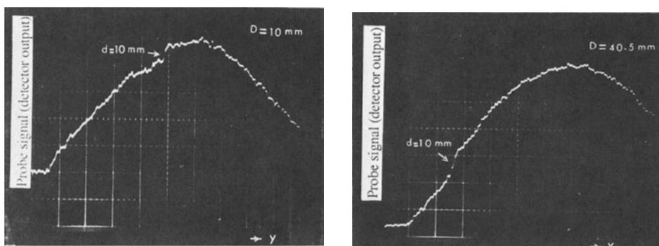
Fig.6 Probe signals about a 10 mm saw-cut notch. Arrows indicate discontinuities in signals.
