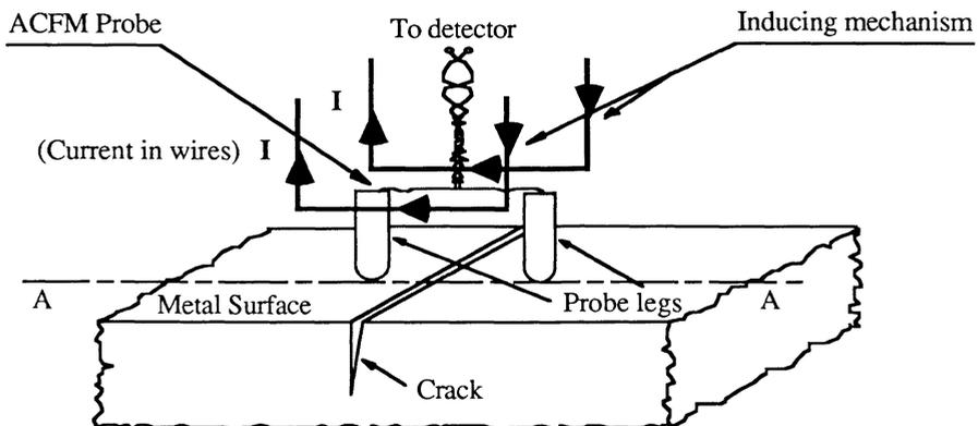
Fig. 1 ACFM probe together with a two-wire inducing mechanism.
