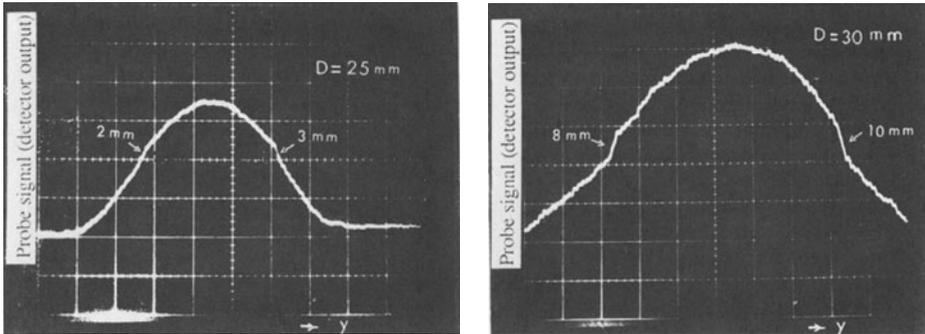
Fig. 7 Probe signals about four saw-cut notches. In these tests, each pair of notches is located symmetrically with respect to the inducing mechanism.
