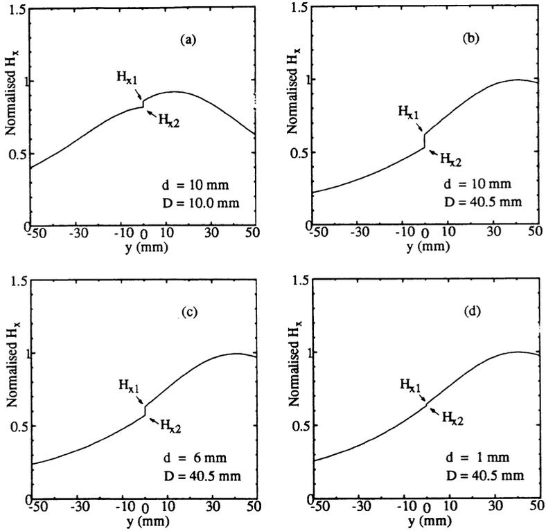
Fig. 4 Theoretical behaviour of induced surface magnetic field ( $H_x$ ) along the y-axis for various values of  $d$  and  $D$ . These curves are normalised to the maximum value of  $H_x$  when no crack is present in the metal.
