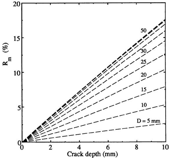
Fig. 5 Variation of  $R_m$  (%) with crack depth for different positions of the inducing mechanism.
