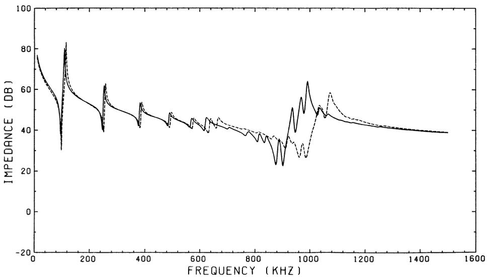
Fig 5 The measured and predicted electrical impedances of a PZT5A disc with a D/T ratio of 10. (\_\_\_\_\_ measurement; ----- finite element prediction)
