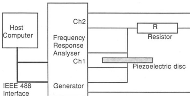
Fig 2. Apparatus used for measurement of the electrical impedance of piezoelectric discs.
