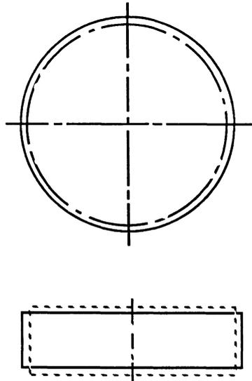
Fig 1. The mode shape of the first through thickness mode of piezoelectric discs assumed by one dimensional analysis.
