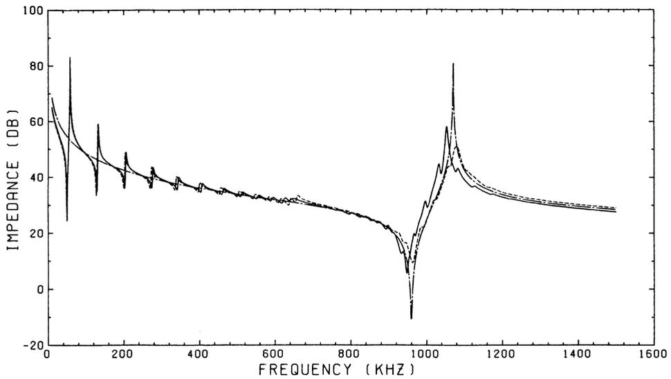
Fig 4 The measured and predicted electrical impedances of a PZT5A disc with a D/T ratio of 20. (\_\_\_\_\_ measurement; ----- finite element prediction; -.-.-.- 1D prediction)
