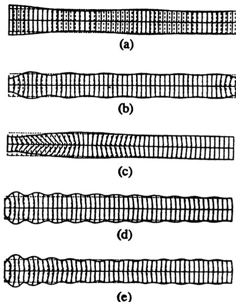
Fig 3 The five types of mode shape of a piezoelectric disc with a D/T ratio of 20.
