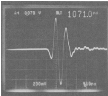
Fig. 3 Typical signal spectra of a 100 MHz transducer made from AlN film.
