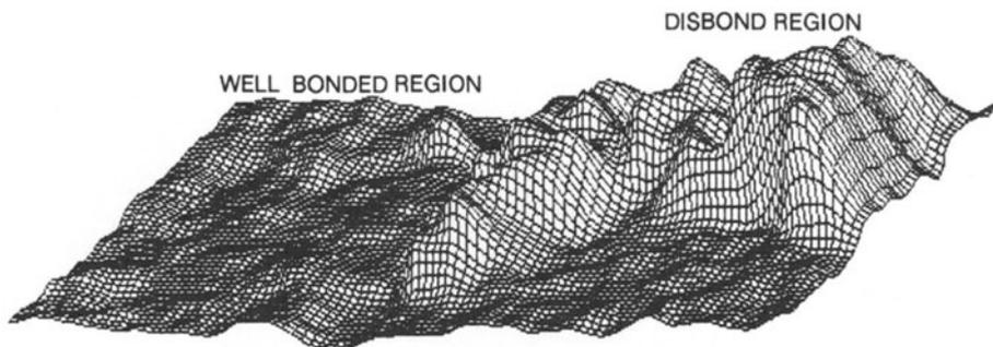
Fig. 2. Ultrasonic Amplitude Image of Disbond Region
