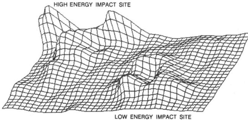
Fig. 4. Ultrasonic Amplitude Image of Two Impact Damage Sites
