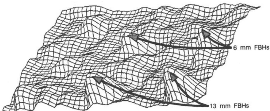
Fig. 3. Ultrasonic Amplitude Image of Flat Bottom Holes
