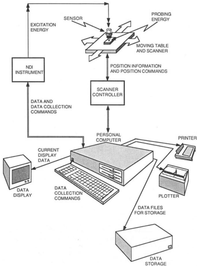
Fig. 1. Nondestructive Inspection System Schematic
