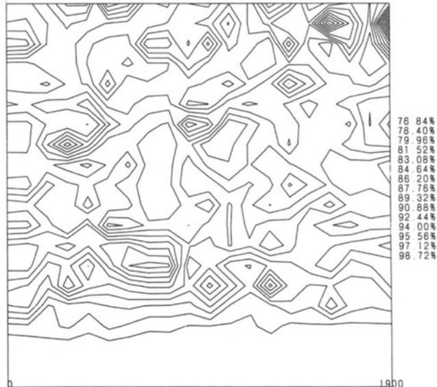
Fig. 3. Contour display of coating on steel surface (Step size: 100 x 100  $\mu\text{m}$ , peak height).
