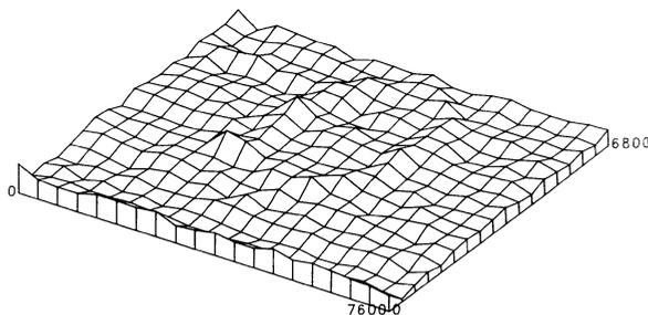
Fig. 8. Axonometric display of photoresist on silicon wafer (Step size: 400 x 400  $\mu\text{m}$ , peak area).
