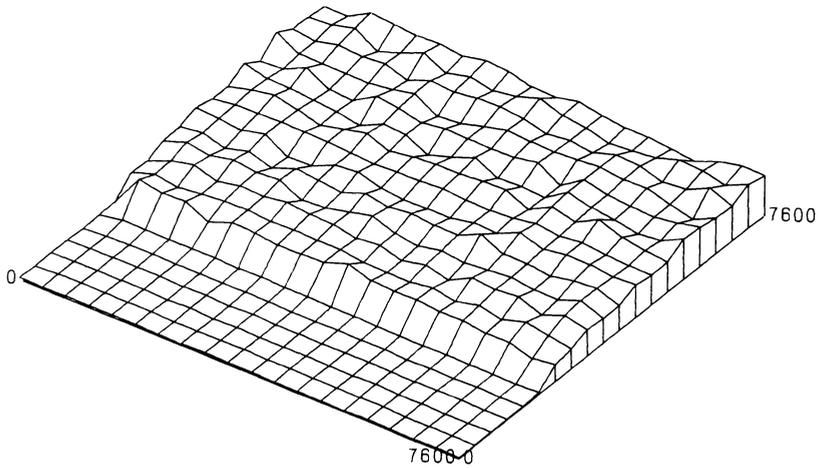
Fig. 2. Axonometric display of coating on steel surface (Step size: 400 x 400  $\mu\text{m}$ , peak height).
