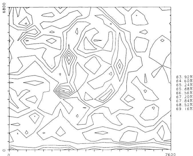
Fig. 7. Contour display of photoresist on silicon wafer (Step size: 400 x 400  $\mu\text{m}$ , peak area).
