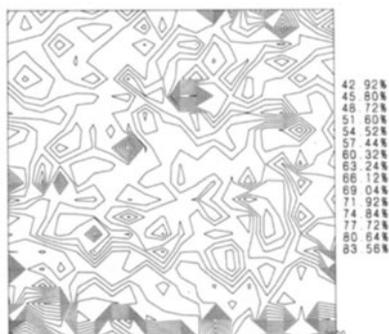
Fig. 5. Contour display of latex coating on paper (Step size: 200 x 200  $\mu\text{m}$ , peak area).
