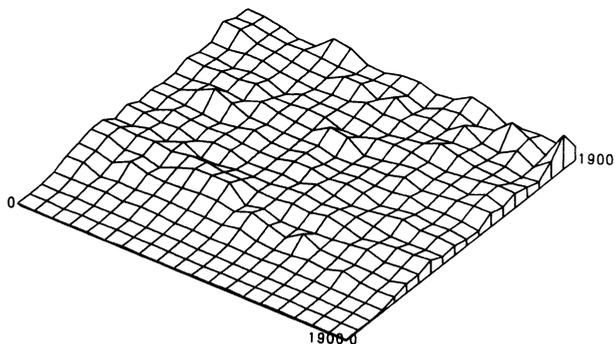
Fig. 4. Axonometric display of coating on steel surface (Step size: 100 x 100  $\mu\text{m}$ , peak height).
