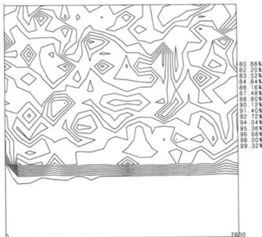
Fig. 1. Contour display of coating on steel surface (Step size: 400 x 400  $\mu\text{m}$ , peak height).
