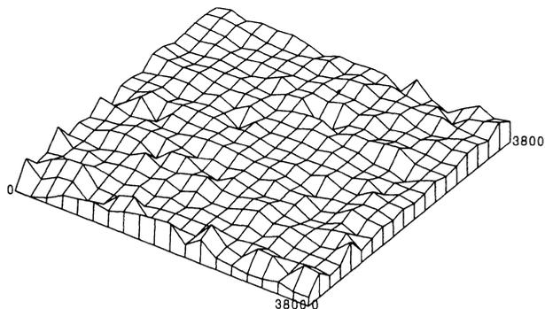
Fig. 6. Axonometric display of latex coating on paper (Step size: 200 x 200  $\mu\text{m}$ , peak area).
