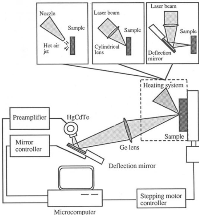
Figure 3. A diagram of the measurement system.
