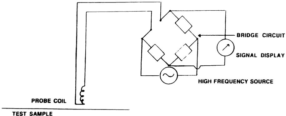
Figure 3. (a) Eddy Current Probe Designs
