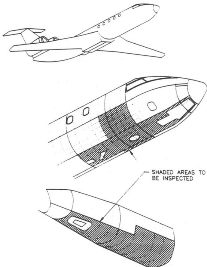
Fig. 1 Typical areas of corrosion requiring eddy current inspection.
