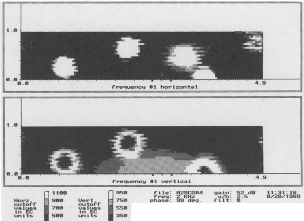
Figure 4. Corroded Stringer Sample (50% wall loss) From Commercial Airliner
