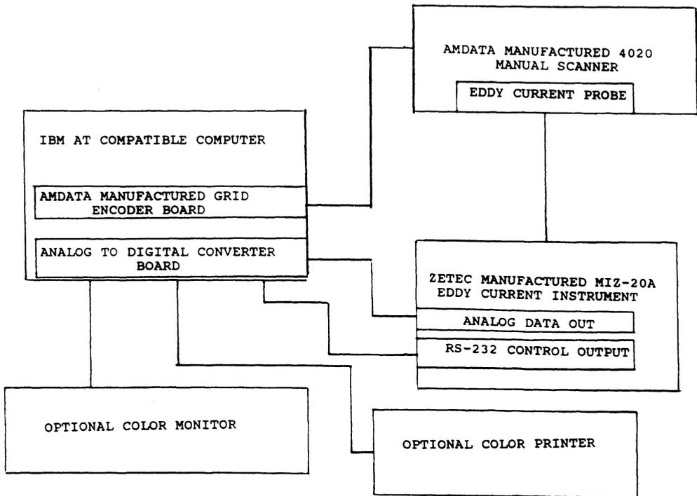
Figure 2. Block Diagram of Laboratory Test System.
