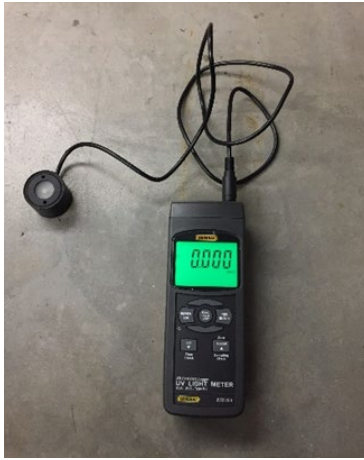
Figure 2 shows a simple UV light meter, UV254SD (General Tools & Instruments LLC., New York, NY, USA), with a plugged-in sensor that can measure either UVA or UVC wavelengths, and it is equipped with a data-logging SD card. As of May 2020, this device sells at a price below $600. Other more advanced devices such as ILT 5000 research/Lab radiometer (International Light Technologies, Peabody, MA, USA) is also available, but it is more expensive (over $1,000). (Photo credit: PL)
