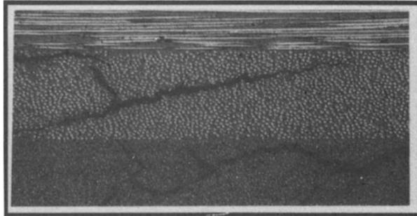
Figure 3. Microstructural damage produced by impact loading.
