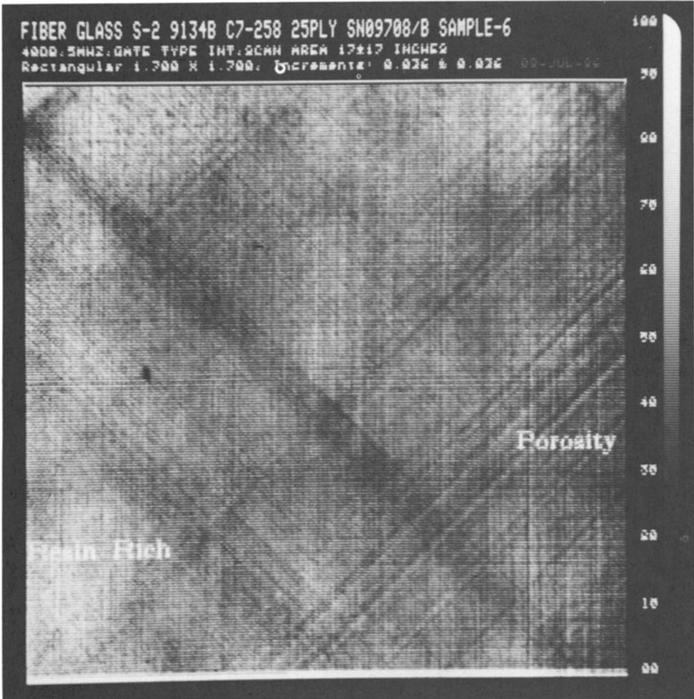
Figure 1. Example of ultrasonic C-scan on 18" x 18" composite panel.
