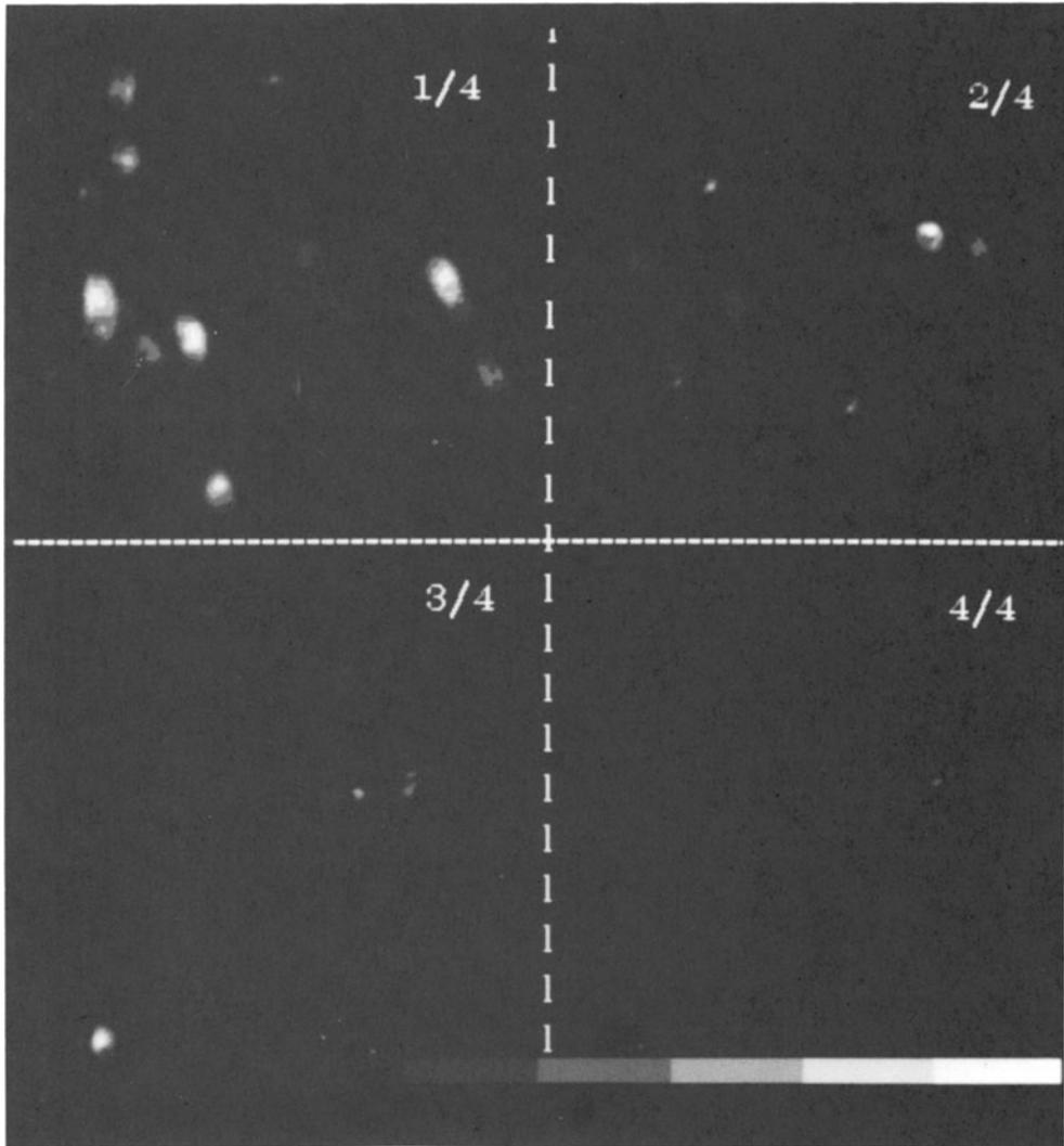
Figure 4. Four ultrasonic C-scans of same impact damaged specimen. Each image displays damage at different depth in plate.
