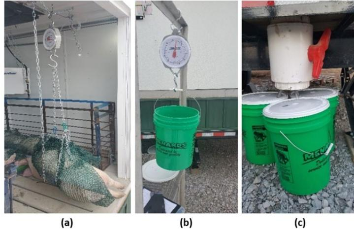
Figure 1. (a) Daily carcass weighing in the rooms using a hanging scale. (b) Daily leachate weighing from leachate collection systems. (c) Leachate collection buckets routed from each carcass bin and through the pit and leachate release valve.
