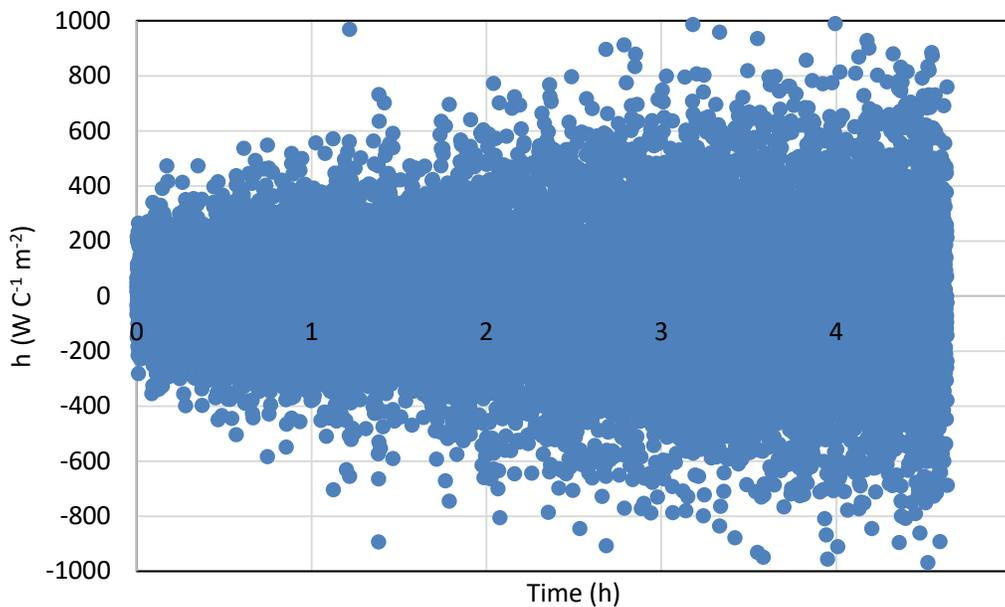
**Figure 3. Raw values for  $h$ , the heat transfer coefficient of the slats, calculated at 1 s time steps.**
