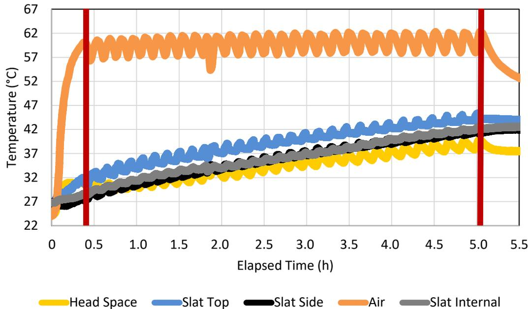
Figure 2. Temperature data collected during the heating event. A subset of data from 0.45 to 5.08 h (shown inside vertical bars) was used for subsequent calculations. Variation in temperature are due to the heater cycling on and off to maintain set point.
