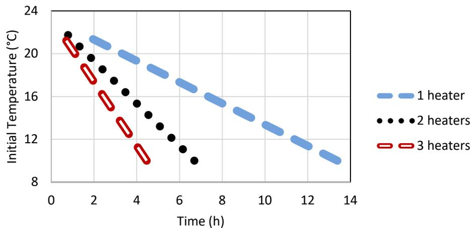
Figure 4. Time required for slats to reach the desired setpoint of  $23.3 \text{ }^\circ\text{C}$  for a range of initial temperatures. Values are shown for a typical 2400 hd,  $84 \times 21.3 \times 2.3 \text{ m}$  finishing barn, assuming a single heater capacity is  $733 \text{ kW}$  ( $250 \text{ kBtu h}^{-1}$ ).
