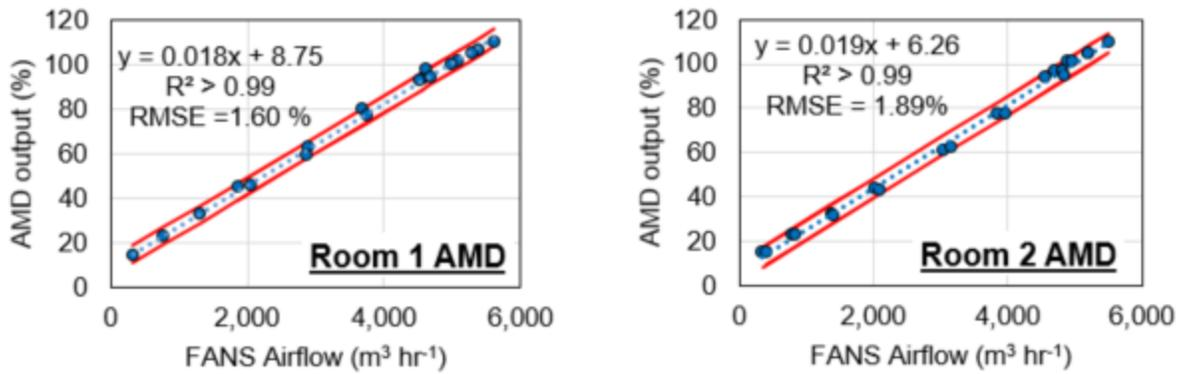
Figure 1. Calibrations for Room 1 and 2 AMD devices against the FANS unit. The red lines represent a 95% prediction interval.
