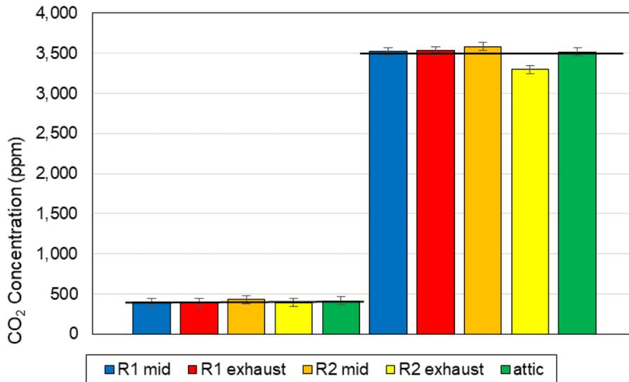
Figure 2. Comparison of the five CO<sub>2</sub> sensors to the span gases. All sensors were within the ±10.0% margin of error of the gas concentration, black lines represent the span gas concentration. The error bars represent the 50 ppm accuracy of the sensors.
