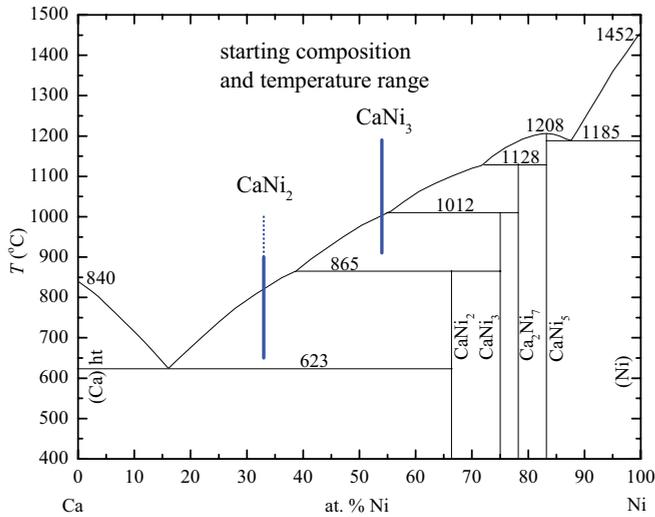
FIG. 1. (Color online) Ca-Ni phase diagram after Notin *et al.* (Ref. 7). Starting compositions and temperature profile for  $\text{CaNi}_2$  and  $\text{CaNi}_3$  growths shown with blue lines (the dotted line represents rapid cooling).
