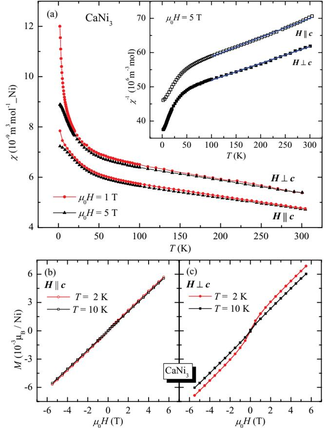
FIG. 5. (Color online) (a) Magnetic susceptibility  $\chi = M/H$  of  $\text{CaNi}_3$  per mol Ni. The moderate increase of  $\chi(T)$  under cooling from 300 K to  $T \approx 20$  K is followed by a significant increase at lower temperatures. The inset shows the inverse susceptibility. Magnetization  $M(H)$  as a function of field for  $H \parallel c$  (b) and  $H \perp c$  (c) at  $T = 2$  and 10 K.
