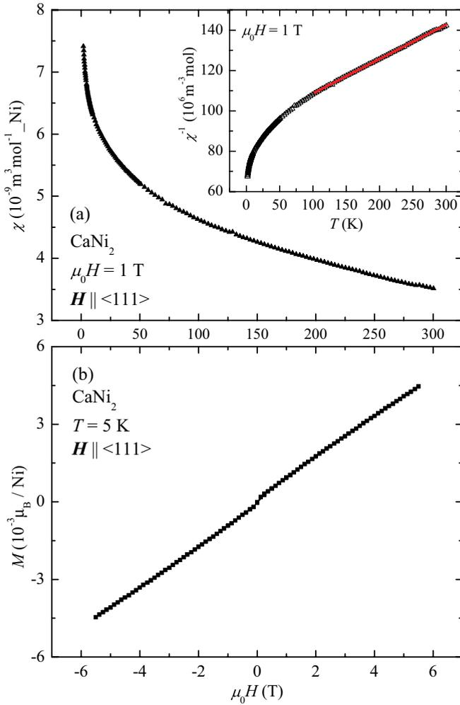
FIG. 4. (Color online) (a) Magnetic susceptibility  $\chi = M/H$  per mol Ni of  $\text{CaNi}_2$ . The moderate increase of  $\chi(T)$  under cooling from 300 K to  $T \approx 20$  K is followed by a significant increase at lower temperatures. The inset shows the inverse susceptibility. (b) Magnetization  $M(H)$  as a function of field.
