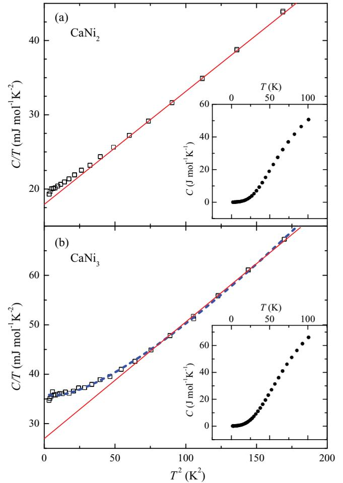
FIG. 7. (Color online) Specific heat plotted as  $C/T$  vs  $T^2$  for (a)  $\text{CaNi}_2$  and (b)  $\text{CaNi}_3$ . Additional contributions to the specific heat of an ordinary metal ( $C/T = \gamma + \beta T^2$ , indicated by the red lines) are observed below  $T \approx 10$  K. Assuming a contribution of spin fluctuations of the form  $C_{\text{mag}} = AT^3 \ln(T/T_{\text{SF}})$  leads to a  $T$  dependence shown by the dashed blue line. Insets: specific heat as a function of temperature.
