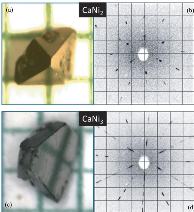
FIG. 2. (Color online) (a)  $\text{CaNi}_2$  single crystal on a millimeter grid and (b) corresponding x-ray Laue back-reflection pattern. (c)  $\text{CaNi}_3$  single crystal on a millimeter grid and (d) corresponding x-ray Laue back-reflection pattern. Both diffraction patterns show the threefold rotation symmetry of  $\{111\}$  and  $\{001\}$  directions of their cubic and hexagonal unit cells, respectively.
