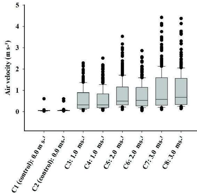
**Figure 4.** Boxplot of air velocity measurements at 275 locations in two replicate cages in still air and 3 controlled velocities. C1 and C2) Control (cages 1 and 2, still air),  $0 \text{ m s}^{-1}$ ; C3 and C4) Cages 3 and 4, set point  $1 \text{ m s}^{-1}$ ; C5 and C6) Cages 5 and 6, set point  $2 \text{ m s}^{-1}$ ; C7 and C8) Cages 7 and 8, set point  $3 \text{ m s}^{-1}$ .
