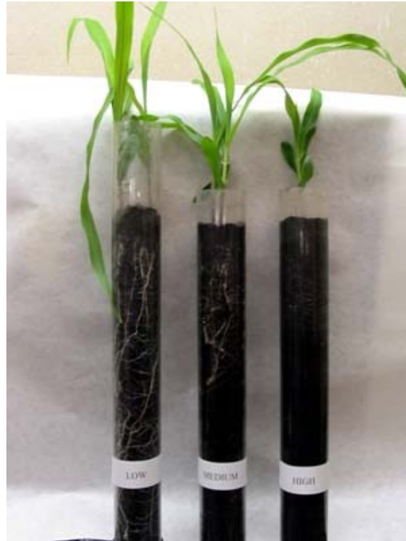
Photo 1. Effect of soil compaction on root growth at three different soil bulk densities: Low, 0.7 g/cm 3 ; Medium, 1.1 g/cm 3 ; High, 1.6 g/cm 3 .
