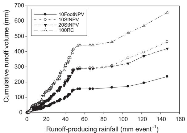
Fig. 4. Cumulative runoff sorted by rainfall event size (mm) for the 3 years studied (April–October). Each point represents the average of the three watersheds for each treatment (10FootNPV, 10StNPV, 20StNPV and 100RC).
