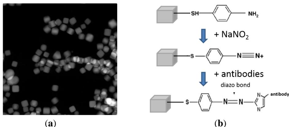
Silver nanocubes were synthesized following the method of Skrabalak *et al.* [26]. Typically, in 20 mL glass reaction vial, 6 mL of ethylene glycol were added. The vial was incubated at  $150\text{ }^\circ\text{C}$  for 1 h to evaporate the water in the system. After heating,  $70\text{ }\mu\text{L}$  of 3 mM  $\text{Na}_2\text{S}$  in ethylene glycol
