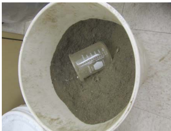
Figure 4. Powdered filamentous algae after hammermill processing
