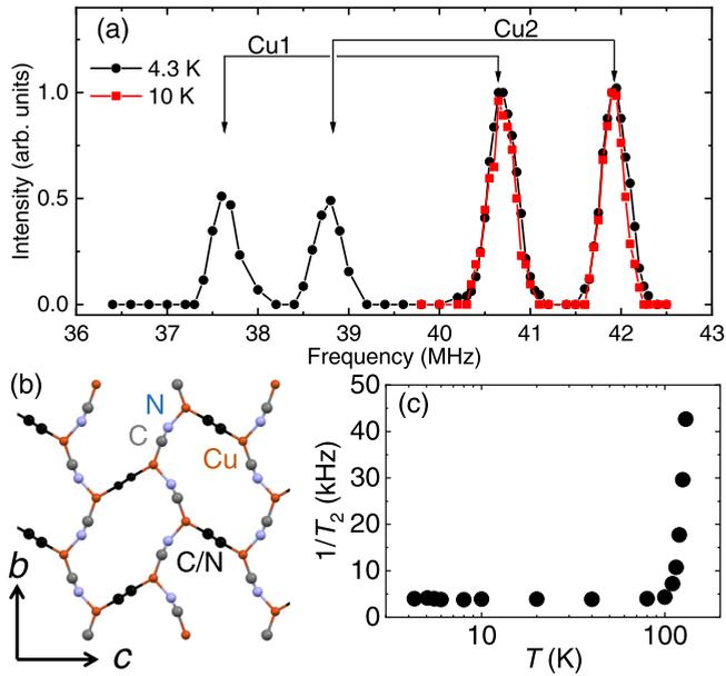
FIG. 1. (a) ZF NQR spectra at 4.3 K (black circles) and 10 K (red squares). (b) Structure of the Cu<sub>2</sub>(CN)<sub>3</sub> insulating layer. (c)  $T$  dependence of  $T_2^{-1}$  measured at the peak around 40.7 MHz.
