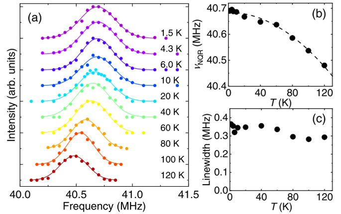
FIG. 2. (a)  $T$  evolution of NQR spectra. Solid lines are the fitting curves using the Gaussian function. (b)  $T$  dependence of  $\nu_{\text{NQR}}$ . The dashed curve is the calculated result with the empirical formula  $\nu_{\text{NQR}} = \nu_0 \exp(-\alpha T^2)$  (see text). (c)  $T$  dependence of the linewidth.
