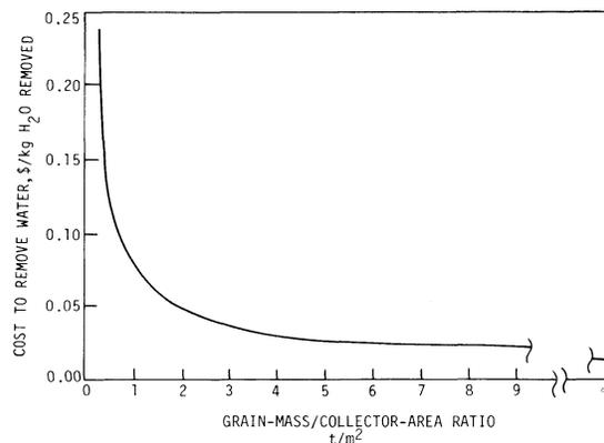
**Fig. 13—**Cost to remove water vs. grain-mass/collector-area. Airflow rate: 0.014 m<sup>3</sup>/s·t (central Iowa).
