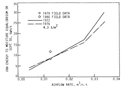
Fig. 8—Electrical energy for fan operation per unit grain mass vs. airflow rate for a grain mass/collector-area ratio of 4.3 t/m<sup>2</sup> (central Iowa).
