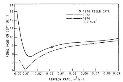
Fig. 5—Final grain moisture content vs. airflow rate for grain-mass/collector-area ratio of 1.2 t/m<sup>2</sup> (central Iowa).
