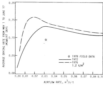
Fig. 3—Average drying rate vs. airflow rate for a grain-mass/collector-area ratio of 1.2 t/m<sup>2</sup> (central Iowa).
