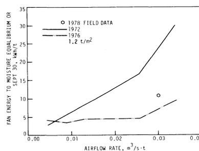
Fig. 7—Electrical energy for fan operation per unit grain mass vs. airflow rate for a grain-mass/collector-area ratio of 1.2 t/m<sup>2</sup> (central Iowa).
