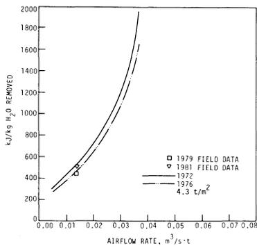
**Fig. 10—**Electrical energy for fan operation per unit of water removed for a grain-mass/collector-area ratio of 4.3 t/m<sup>2</sup>. Grain depth = 4.6 m (central Iowa).
