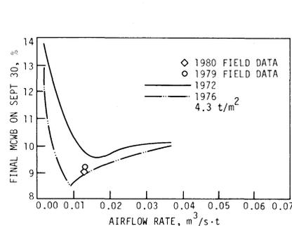
Fig. 6—Final grain moisture content vs. airflow rate for grain-mass/collector-area ratio of 4.3 t/m<sup>2</sup> (central Iowa).
