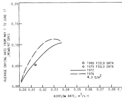
Fig. 4—Average drying rate vs. airflow rate for a grain-mass/collector-area ratio of 4.3 t/m<sup>2</sup> (central Iowa).
