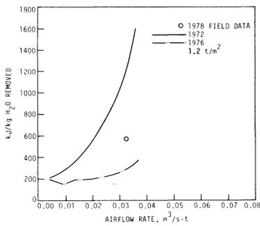
**Fig. 9—**Electrical energy for fan operation per unit of water removed for a grain-mass/collector-area ratio of 1.2 t/m<sup>2</sup>. Grain depth: 4.6 m (central Iowa).
